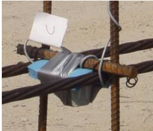
Figure 4-17: iButton attached to a stirrup
