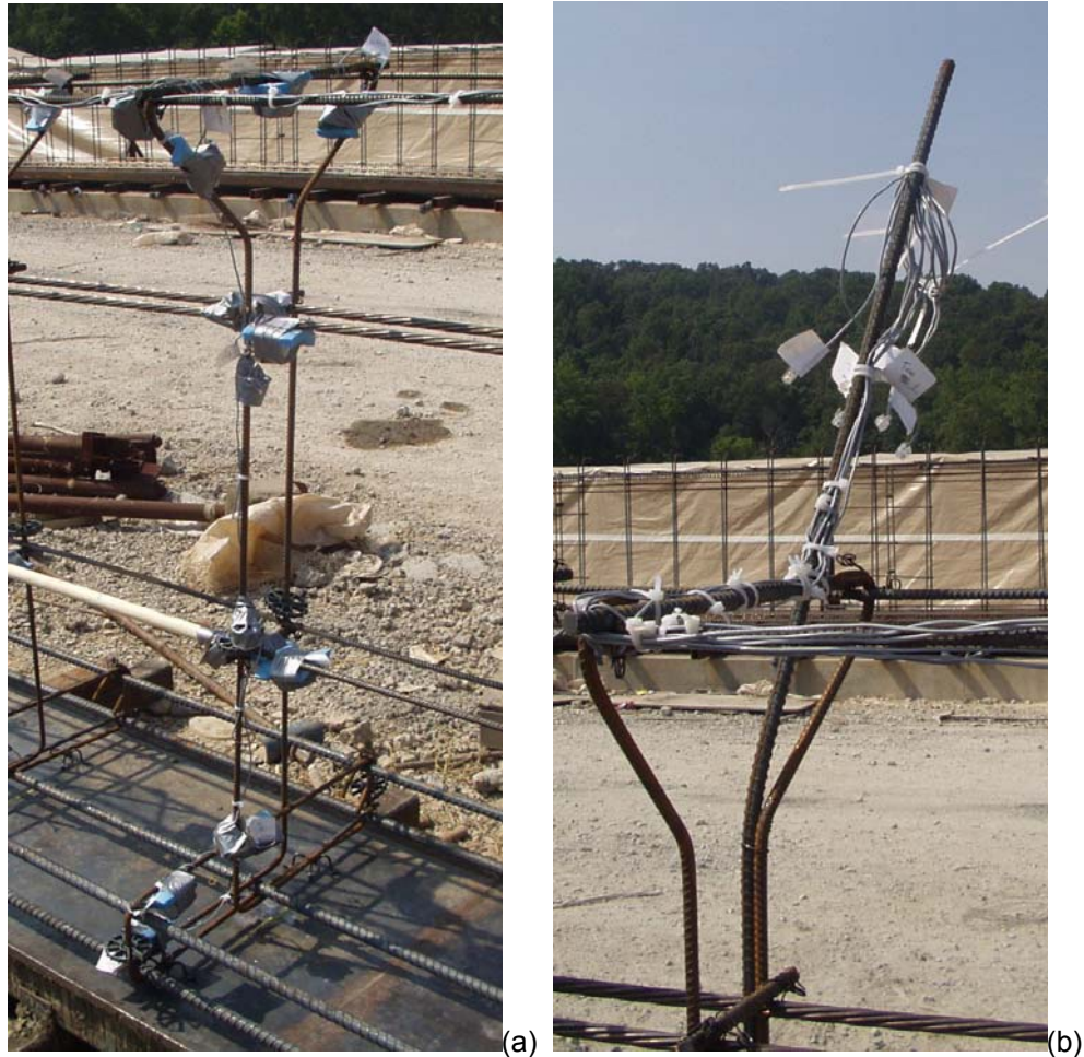
Figure 4-18: (a) iButton Tree 4 installed on a stirrup and (b) Lead wires with phone jacks
