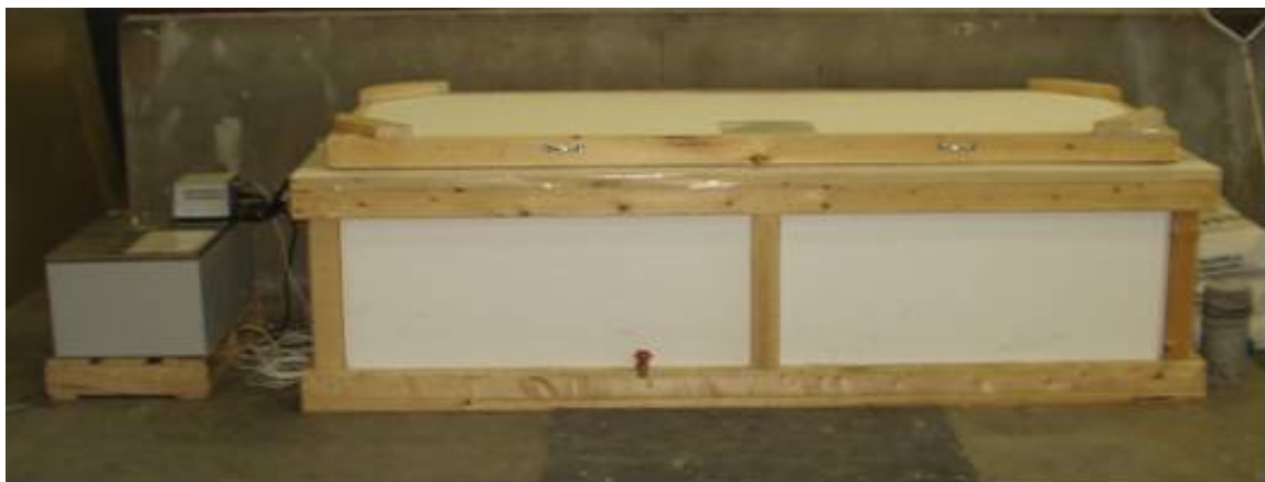
Figure 3-2: Curing tank and programmable heating/cooling circulator
