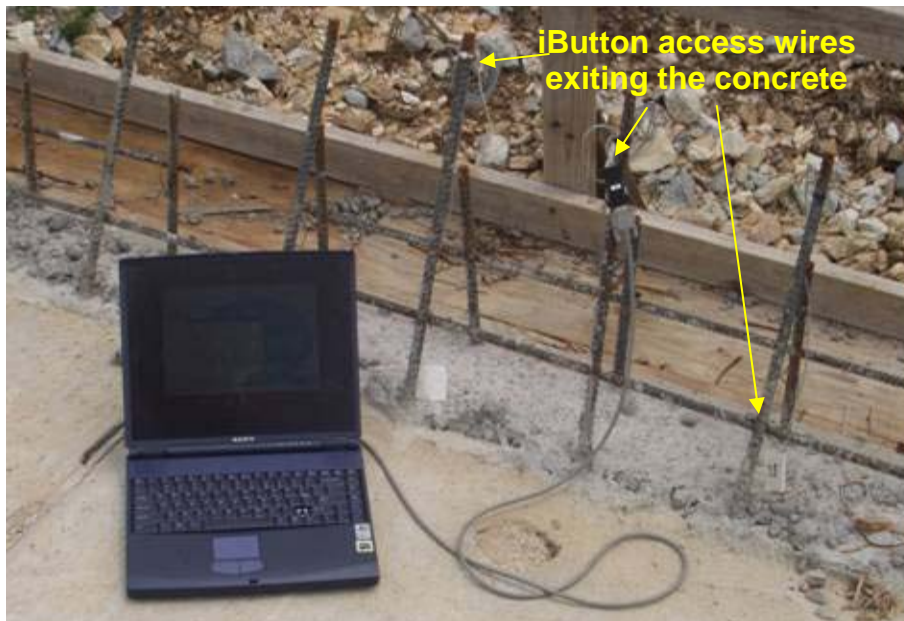
Figure 5-20: iButton wires exiting the concrete
