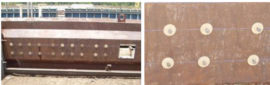
Figure 4-20: Side-mounted pullout inserts on mock girder forms
