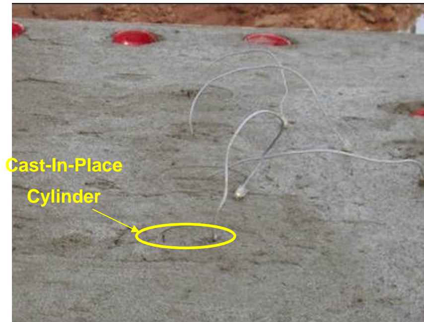
Figure 5-11: iButtons embedded in the cast-in-place cylinders
