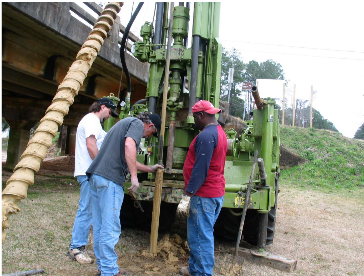
Figure 10. Drilling crew collecting samples at Pea River site at Elba
