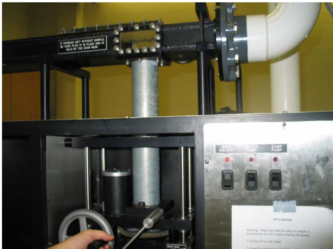
FIGURE 35. Raising the Shelby tube into the conduit opening and placing it flush with the bottom using the crank wheel
