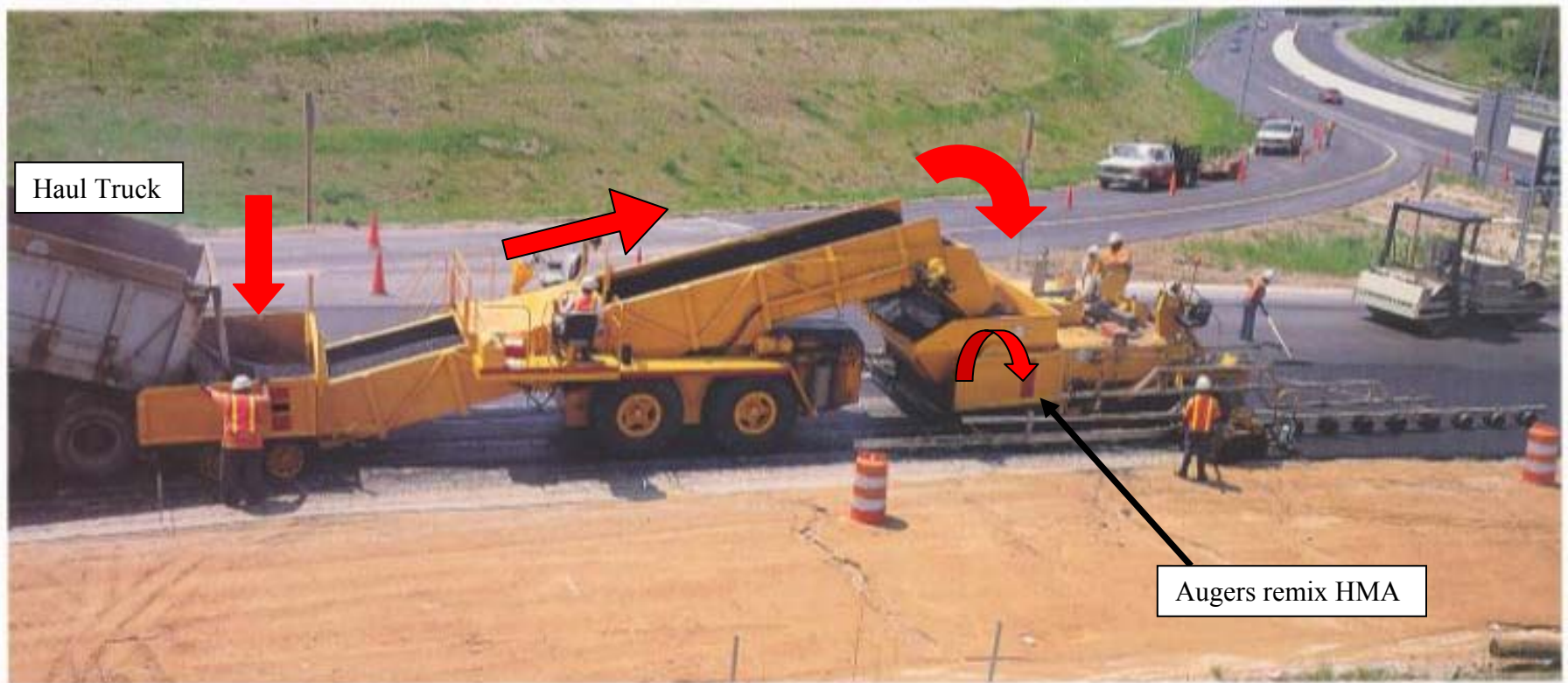
Figure 2. Blaw-Knox MC-330. (The red arrows show the path that the mix follows).
