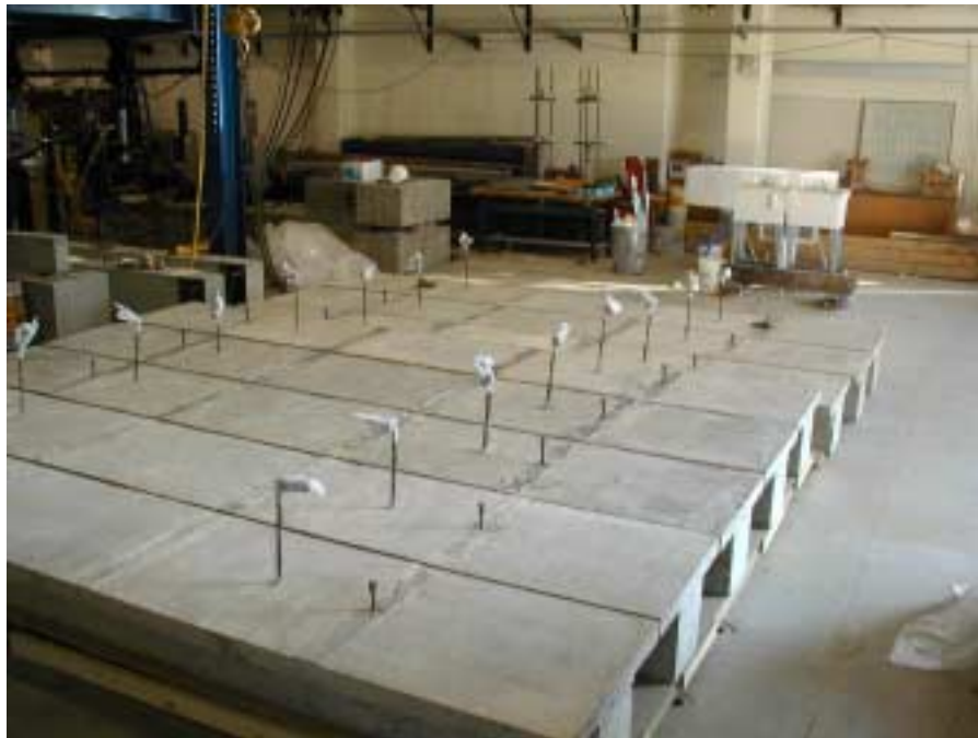
Figure 3.8 Beams after Casting
