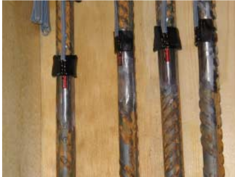
Figure 3.6 Steel Reinforcement Strain Gauges
