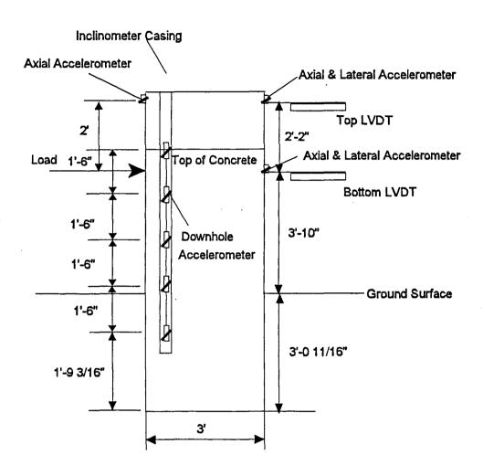
Figure 5 Test Setup, Shaft B6
