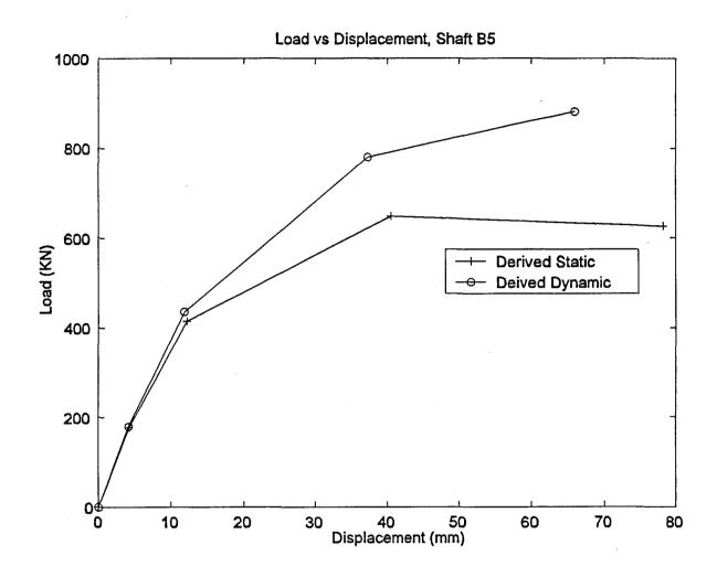
Figure 19 Derived Load Displacement Response, Shaft B5
