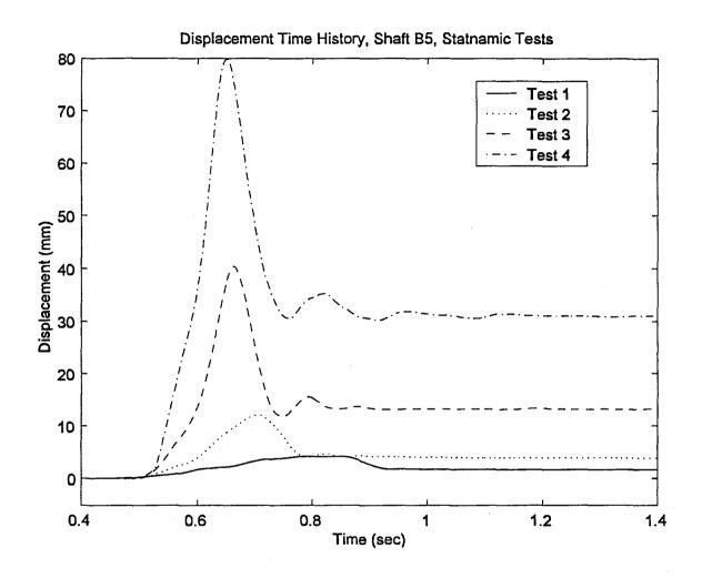
Figure 12 Displacement Time History, Shaft B5
