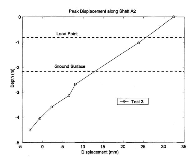
Figure 26 Displacement Profile along Shaft A2
