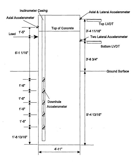
Figure 2 Test Setup, Shaft A2
