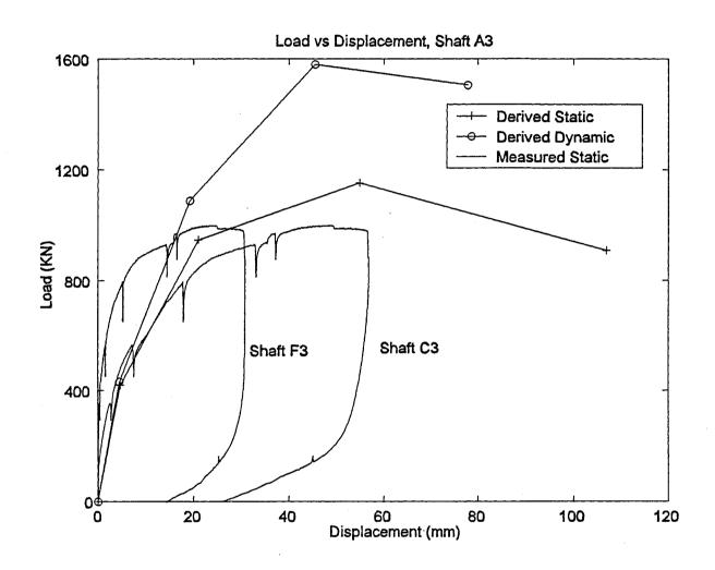
Figure 23 Comparison of Statnamic and Static Test, Shaft A3
