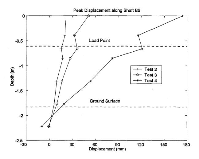
Figure 29 Displacement Profile along Shaft B6
