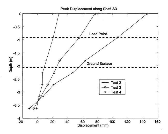
Figure 27 Displacement Profile along Shaft A3
