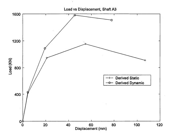
Figure 17 Derived Load Displacement Response, Shaft A3
