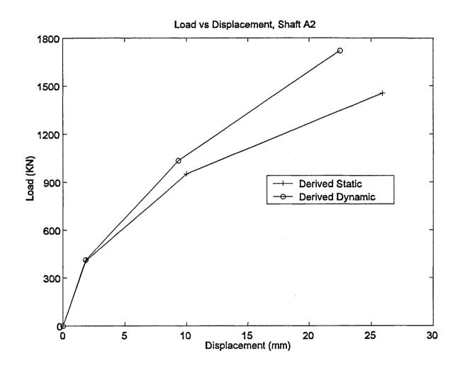
Figure 15 Derived Load Displacement Response, Shaft A2
