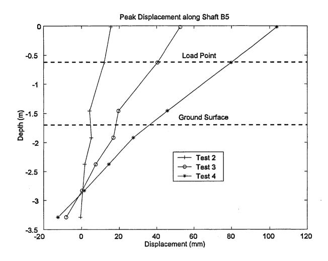
Figure 28 Displacement Profile along Shaft B5
