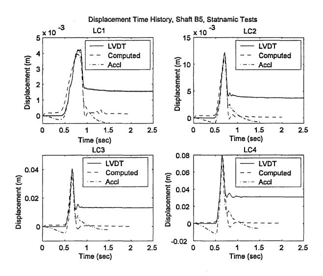
Figure 18 Measured and Computed Displacement Response, Shaft B5
