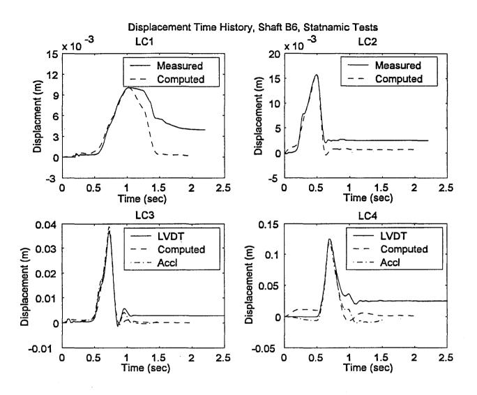
Figure 20 Measured and Computed Displacement Response, Shaft B6
