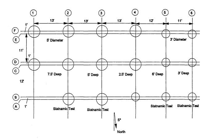
Figure 1 Spring Villa Test Site Layout
