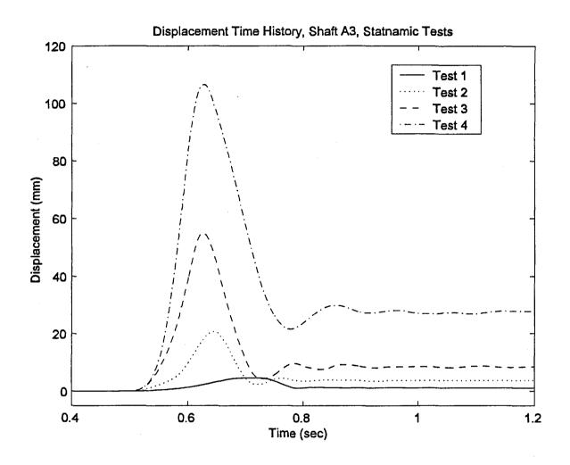
Figure 11 Displacement Time History, Shaft A3
