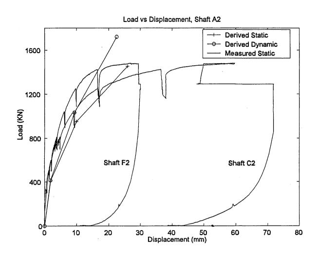
Figure 22 Comparison of Statnamic and Static Test, Shaft A2
