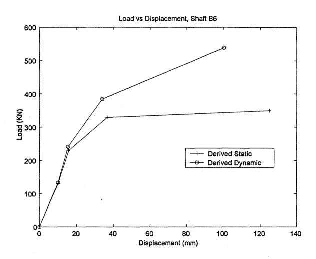
Figure 21 Derived Load Displacement Response, Shaft B6
