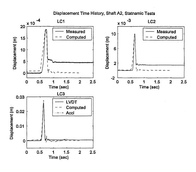
Figure 14 Measured and Computed Displacement Response, Shaft A2
