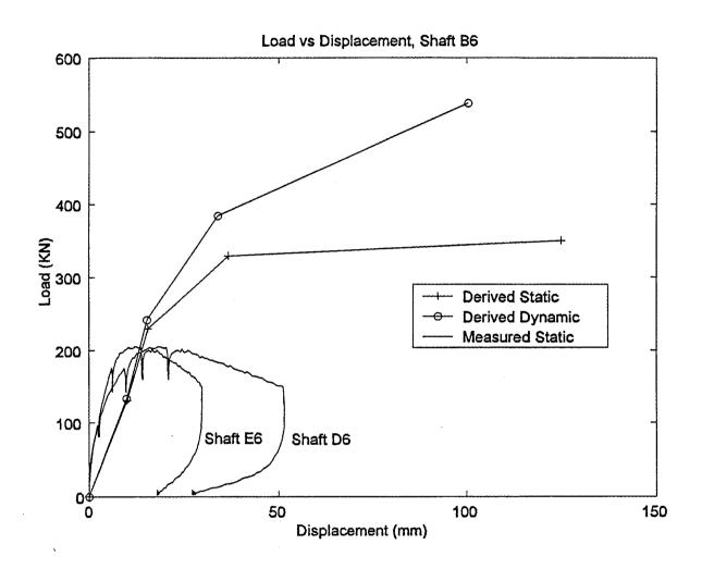
Figure 25 Comparison of Statnamic and Static Test, Shaft B6
