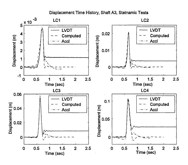
Figure 16 Measured and Computed Displacement Response, Shaft A3
