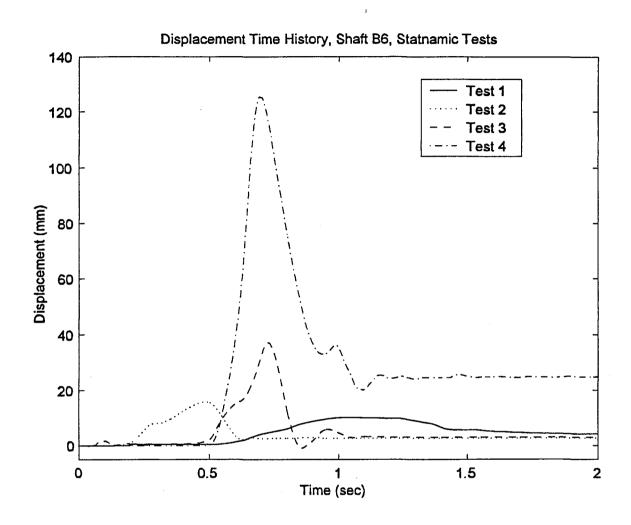
Figure 13 Displacement Time History, Shaft B6
