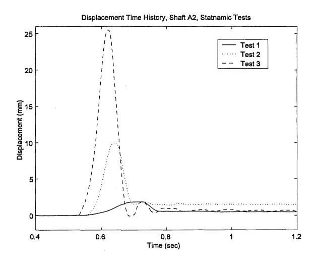
Figure 10 Displacement Time History, Shaft A2
