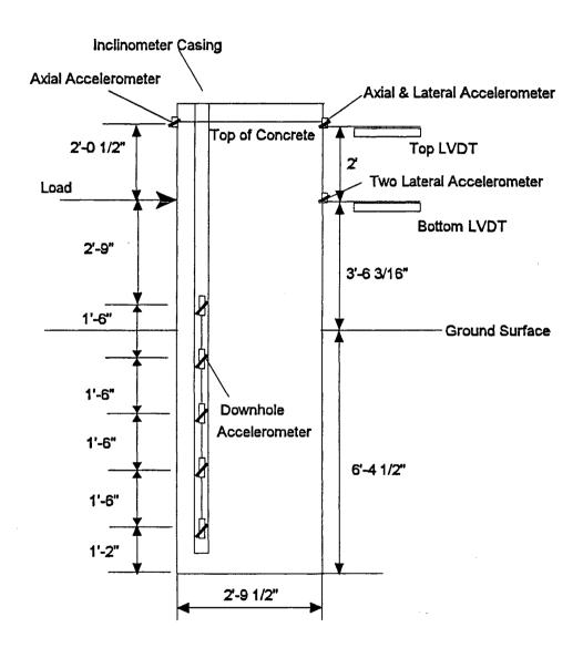
Figure 4, Test Setup, Shaft B5
