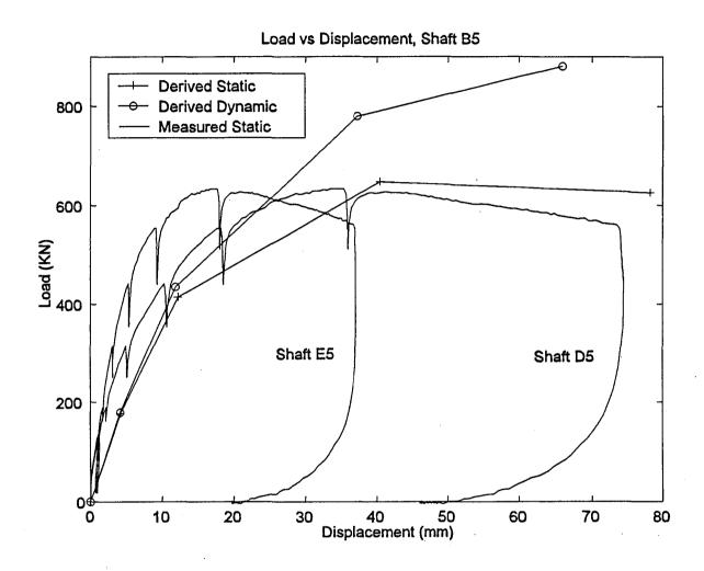
Figure 24 Comparison of Statnamic and Static Test, Shaft B5
