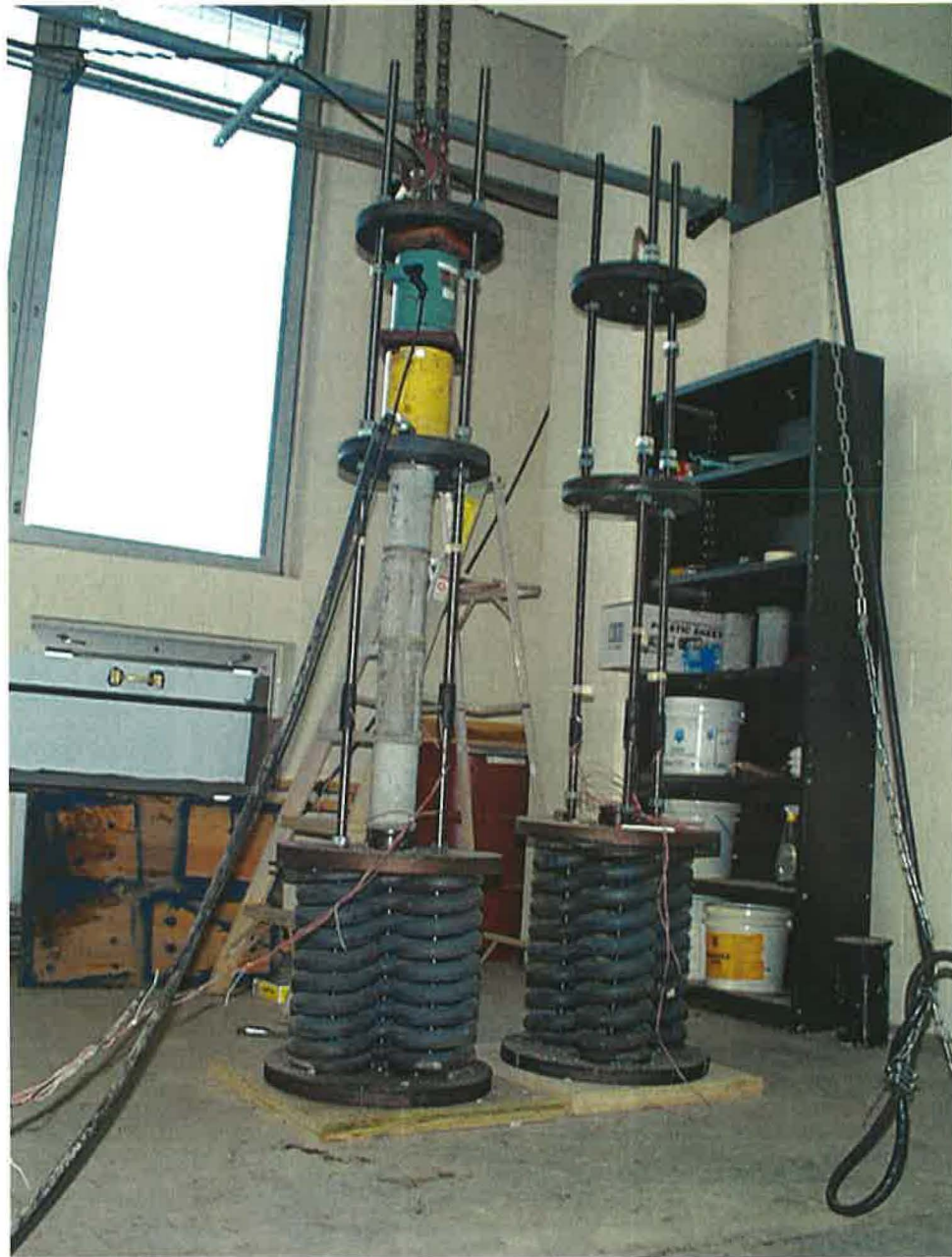
Figure 4.5 Creep Frame Shown with Jack and Load Cell in Place
