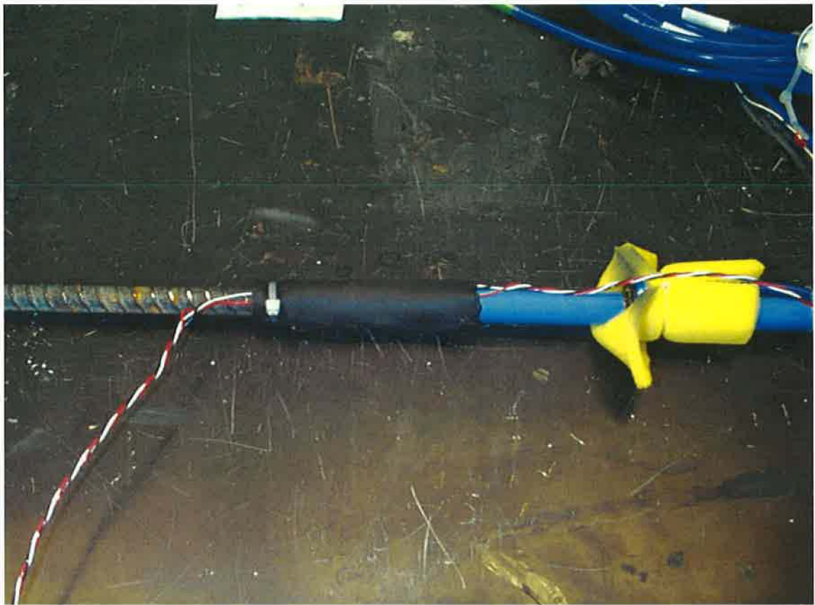
Figure 3.9 Black Waterproofing Material over Electrical Resistance Strain Gages
