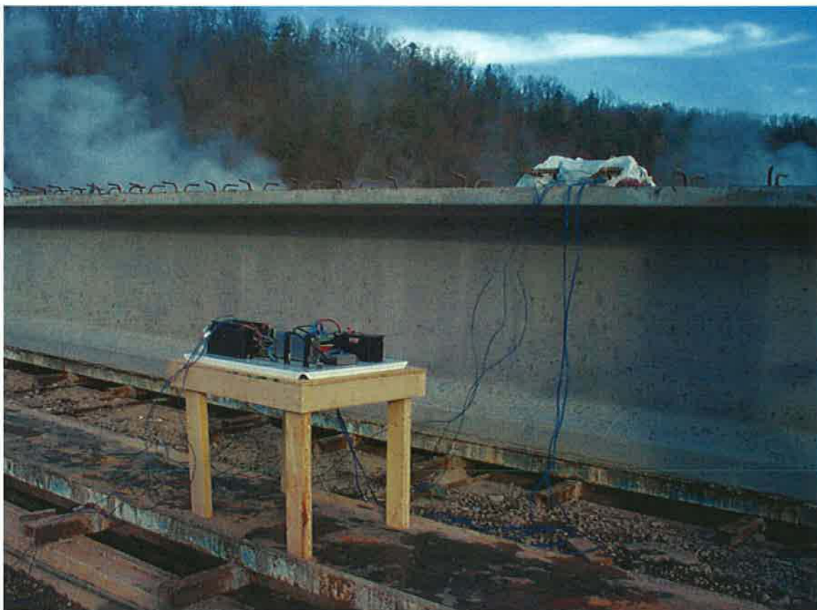
Figure 3.6 CR10X Being Used to Collect Data at Prestressing Yard
