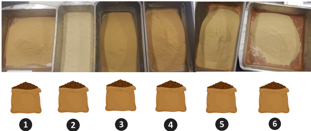
Figure 4.2: Soil colors observed from different bags after oven-drying and sieving
