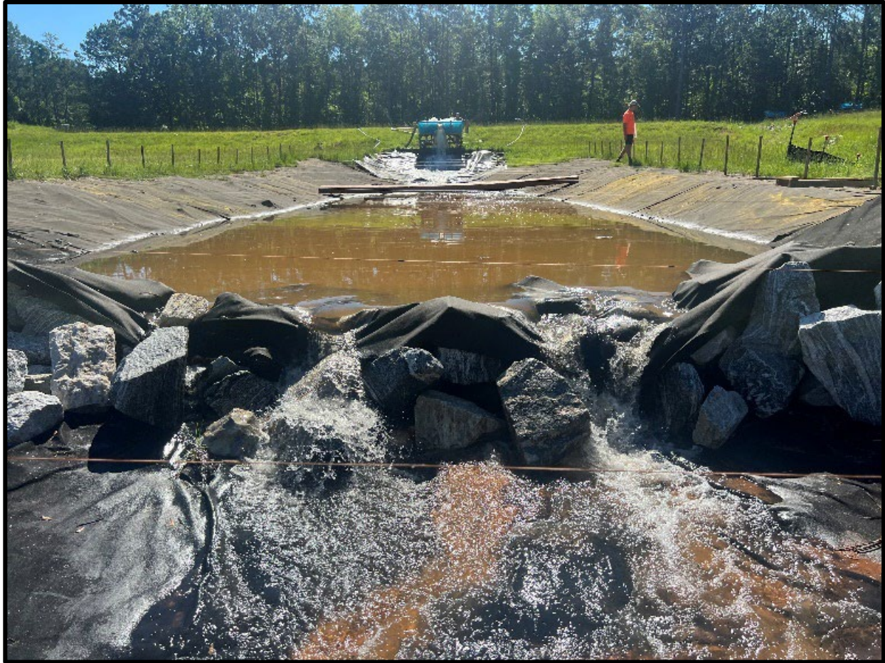
Figure 4.6: Flow Overtopping at Lowest Point Between Large Rocks of M3
