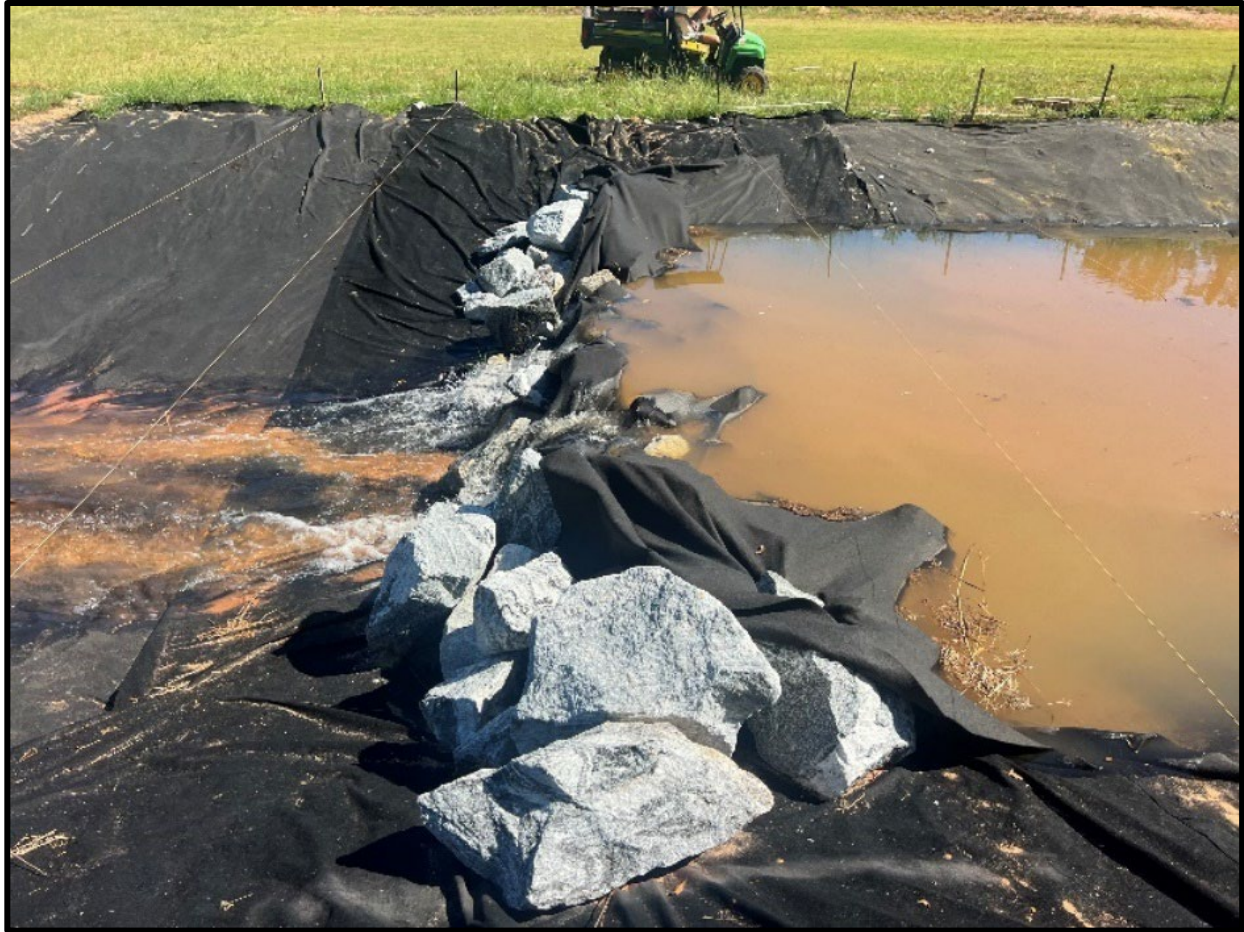
Figure 4.12: High Flow Velocities Downstream of Overtopped Installation
