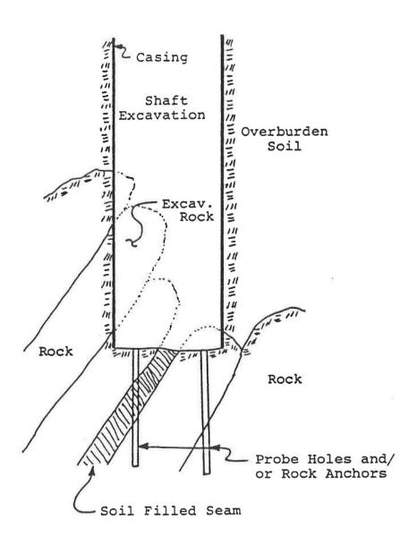
Figure 3. Probe holes and or rock anchors.
