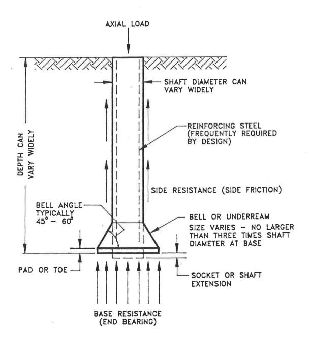
Figure 2. A typical drilled shaft with a bell or underream.
