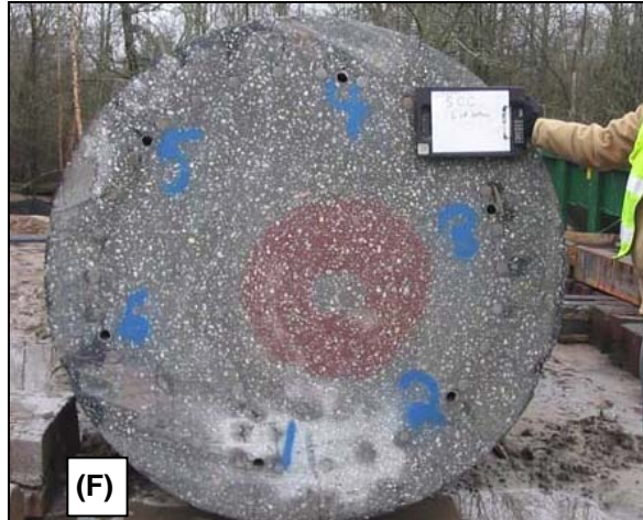
Figure 3: Exhuming and cutting of shafts: (A) Exhuming shaft, (B) Bottom 6 ft of shaft, (C) Wire saw cutting operation, (D) SCC Shaft after first cut, (E) Section of SC Coastal shaft, (F) Section of SCC shaft (6 ft from base)
