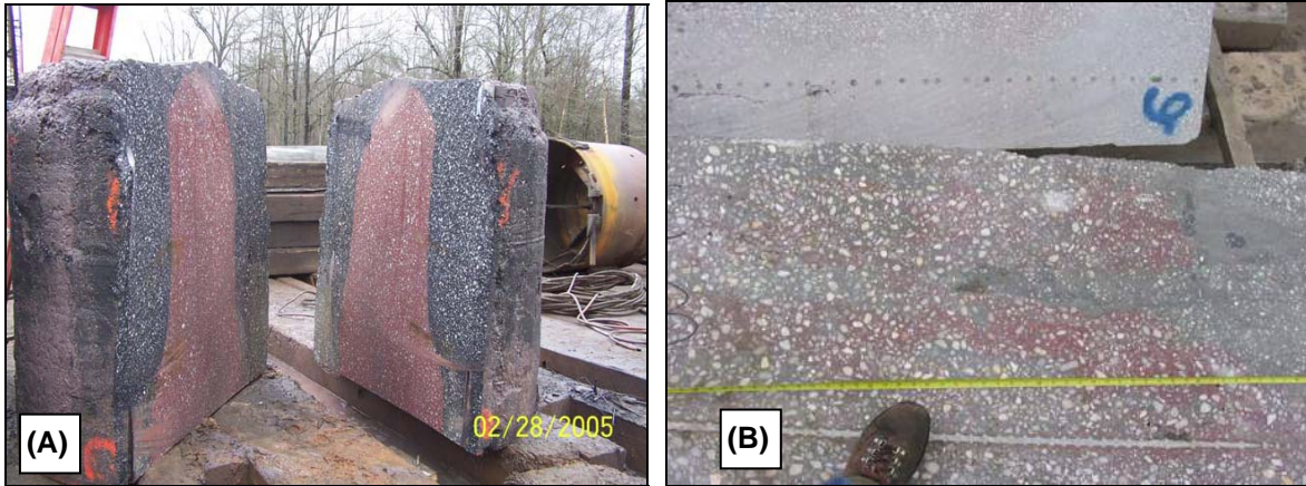
Figure 4: Cut sections of shafts: (A) SC Coastal shaft, view through bottom 6ft (top of photo is bottom of shaft), (B) SCC shaft, View of mixing in upper 13 ft
