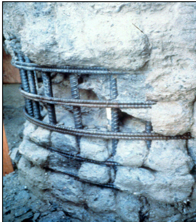
Figure 3.17: Shaft Defects due to the Loss of Workability from Construction Delays (O'Neill and Reese 1999)
