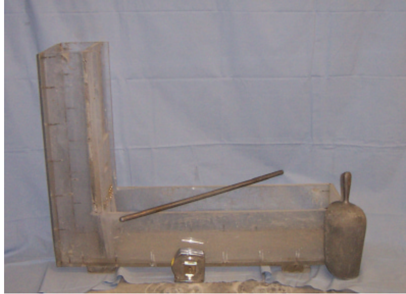
Figure 5.7: Testing Equipment for L-Box Test
