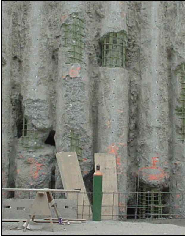
Figure 3.6: Example 1 of Shaft Defects due to the Loss of Workability (photograph courtesy of Dr. Dan Brown)
