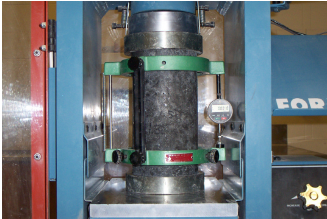
Figure 5.9: Concrete Specimen with Compressometer Attached
