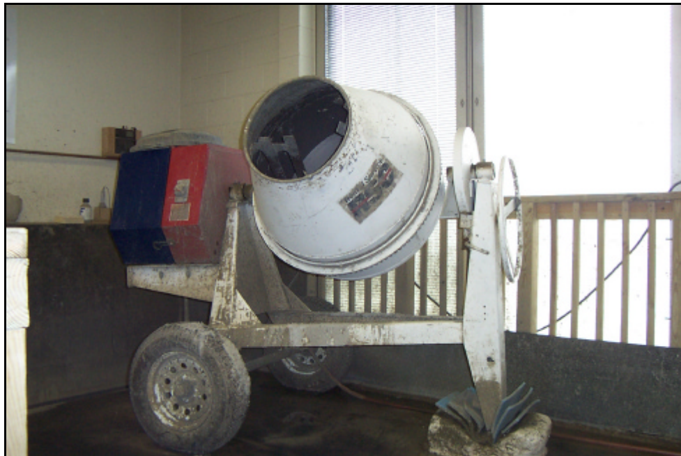
Figure 5.2: 12 ft 3 Concrete Mixer used for this Research
