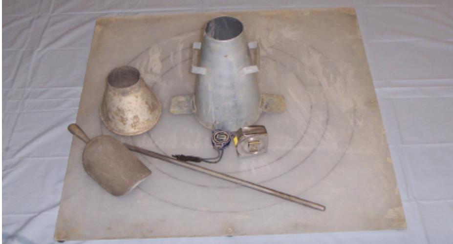
Figure 5.4: Testing Equipment for Slump Flow Test
