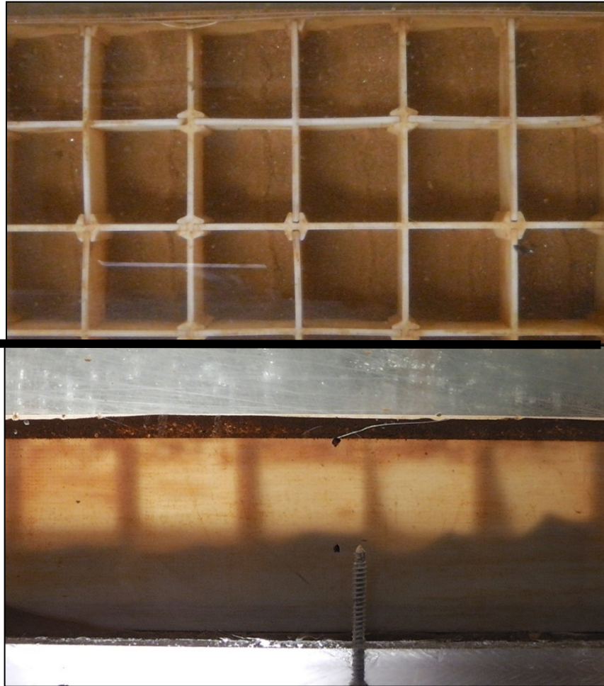
Figure 43 – Post-test configuration H5-W3-50 plan view (top) and profile with backlighting used to illustrate the sediment distribution (bottom)
