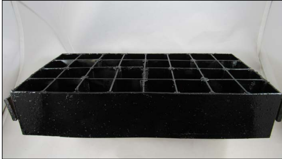
Figure 25 - Horizontal W3-H5 cell configuration with steel weights on ends of cells
