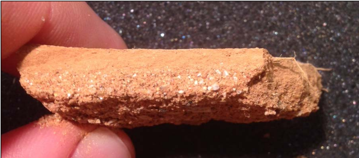
Figure 42 - Dried sediment sample indicating stratification of particles closer to the bottom of the settled sediments
