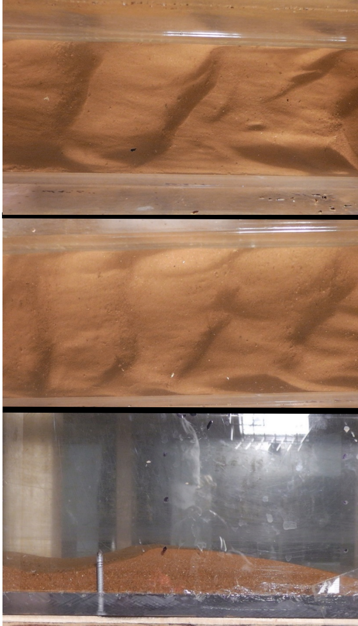
Figure 46 - Unprotected, UP-50 configuration, plan view (top and middle) and profile view (bottom)
