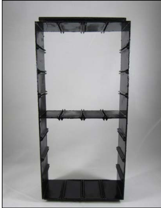
Figure 21 - Confinement cell base, largest cell configuration, W12
