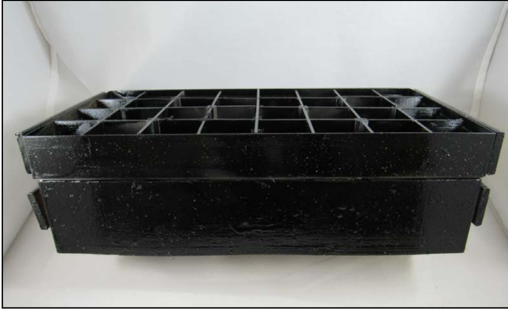
Figure 26 - W3-H8 confinement cell configuration with stacked W3-H5 and W3-H3 cells
