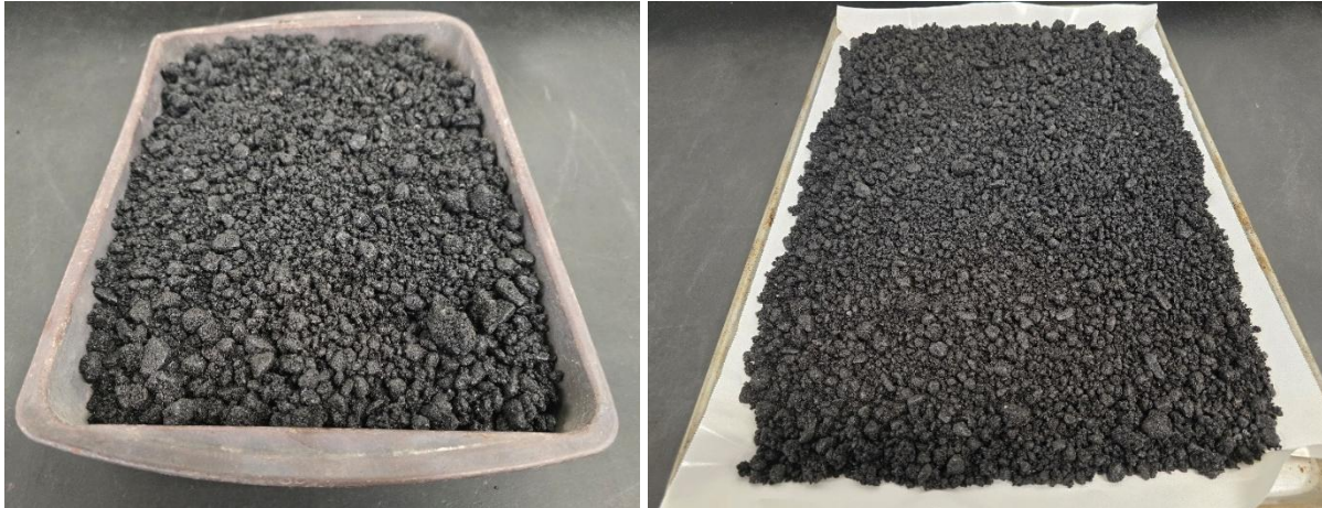
Figure 5. Aging Vessels Used for AASHTO R 121-24 Methods B and D (Left) and Methods C and E (Right)
