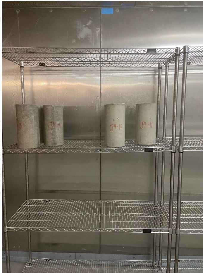
Final Curing 73.5 \pm 3.5 °F and 100% RH
