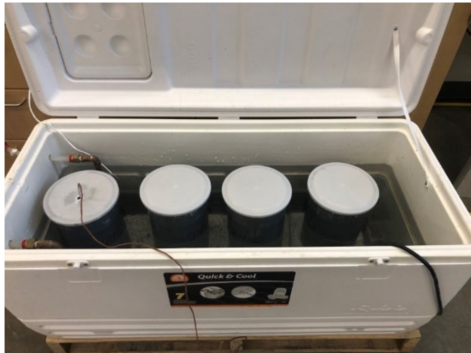
Initial Curing Tank
