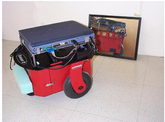
Fig. 14. Pioneer 1 robot with a laptop computer.
