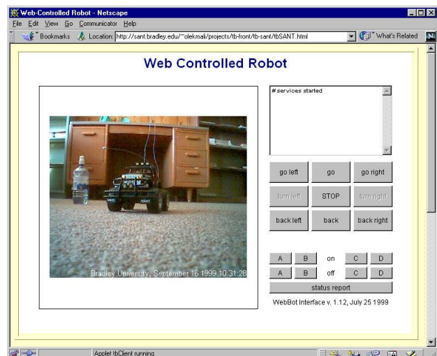
Fig. 5. The web page to control the explorer with the feedback through on side camera.
