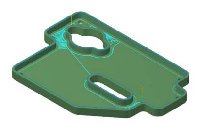
**12** Click **OK** to generate the dynamic rest mill toolpath.
