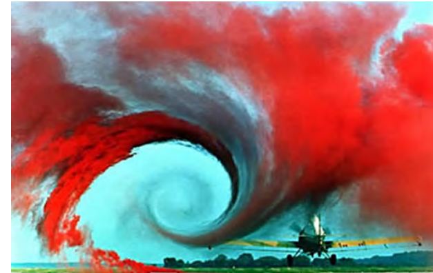
Figure 11. Wingtip vortex turbulence [8]
