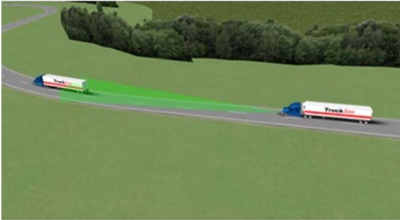
Figure 1: A platoon of two trucks, simulated using TruckSim, traveling on a public highway. This simulation will be adapted to include an EKF for sensor fusion, as well as a controller for the following truck to maintain a constant distance from the lead truck.
