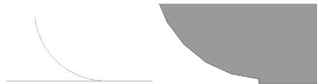
Figure 3. Example of Singularity Changed by Trivial Modification of Geometry
