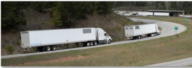
Figure 8. Peterbilt 579 Tractors in Platoon Utilizing Peloton's Prototype DATP System
