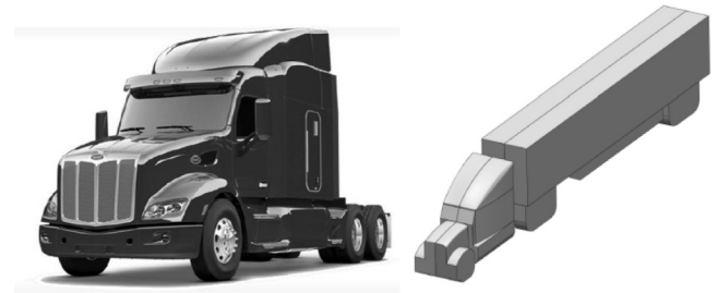
Figure 2. Photo of Peterbilt 579 Cab (provided by Peterbilt) vs. Defeatured Cab and Trailer for Simulation
