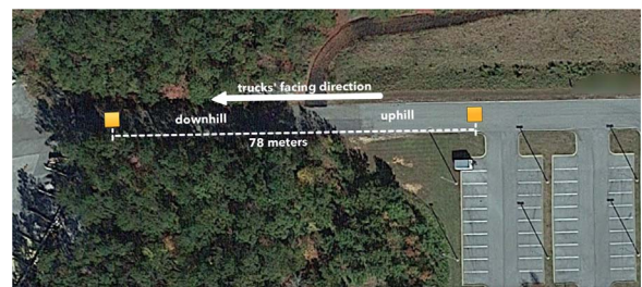
Fig. 5. Static test setup in Location A where a hump is between the trucks.
