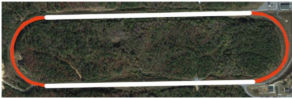
Fig. 10. Test track partition: white straight lines are where messages are marked as “Straight”, and red curves are where messages are marked as “Curve”.
