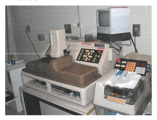
Automated Diving Saw Used to dice a wafer into die
