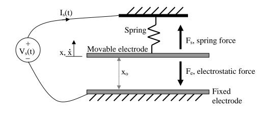
Figure 2.8. An illustration of an electrostatic parallel plate actuator.
