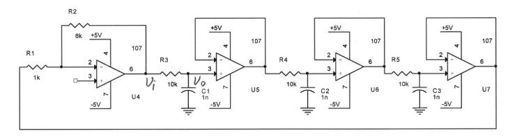
$$\left(\frac{V_0}{V_i} = \tan^{-1}(-RCW) = -60^{\circ} \text{ for oscillation}\right)$$
