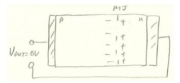
In the presence of light with  $E \ge E_G$ , a non-equilibrium condition exists: holes accumulate on the p-type side of the MJ and electrons accumulate on the n-type side.
