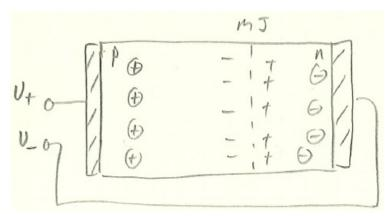
Now a voltage difference exists between the anode and the cathode:  $V_+ - V_- > 0 V$ . Electrons in the p-type Si (minority carrier) flow across the MJ to the n-type Si. Holes in the n-type Si (minority carrier) flow across the MJ to the p-type Si. Therefore, the semiconductor PV device is a <u>minority carrier</u> device.
