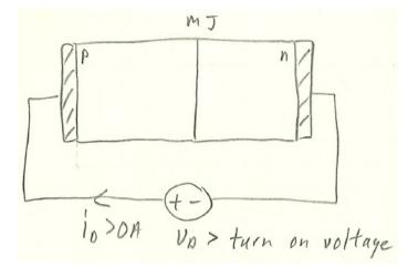
The applied positive voltage, V<sub>D</sub>, reduces the potential barrier:
