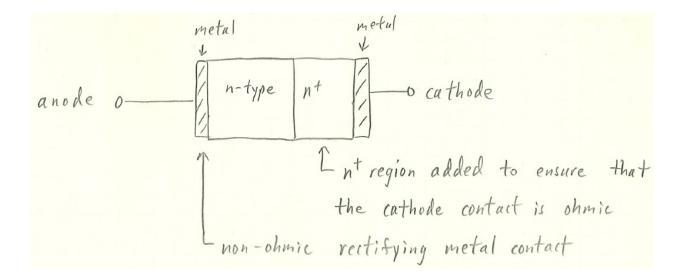
Typically, the Schottky diode has a lower turn-on voltage than a pn junction diode, and switches on and off very fast.
