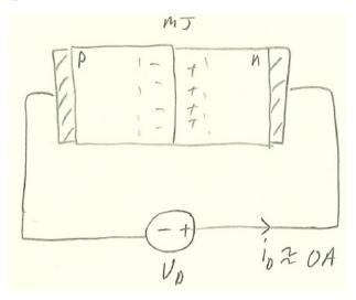
The applied negative voltage,  $V_D$ , increases the potential barrier to a net of charge carriers moving across the MJ:  $i_D \approx 0A$ .
