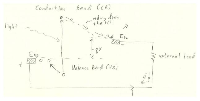
Light of sufficient energy creates and electron-hole pair (i.e. an electron moves to the CB).
