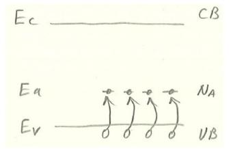
$E_v$  is so close to  $E_a$  that almost all acceptor sites are filled, leaving holes in the valence band for conduction.
