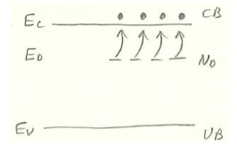
$E_D$  is so close the  $E_C$  that almost all electrons at  $E_D$  have moved to the CB and are available for conduction.
