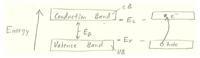
In the drawing above, an electron-hole pair is created when an electron moves from the valance band to the conduction band. For example, due to thermal energy. The electron cannot have an energy level between  $E_c$  and  $E_v$ .
