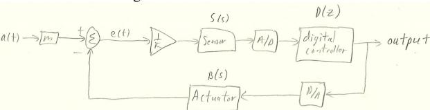
The digital controller can be implemented on a microcontroller in software or in programmable logic circuitry (FPGA, PLA, etc.). An advantage of this implementation is that the digital controller can easily be modified by changing the programming.
