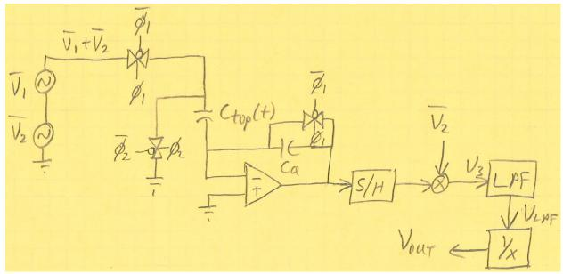
This interface / PPA drive circuit is for one side only. The other side (other PPA) would have a similar circuit.  $C_{top}(t)$  and  $C_a$ , along with the AC analog switches (little triangles with the dot and the  $\emptyset$  and  $\overline{\emptyset}$  drive signals) form a charge amplifier with the input signals being  $\sim$ AC. Actually,  $\overline{V}_1$  is really time varying DC, while  $\overline{V}_2$  is single frequency AC.
