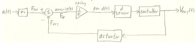
$F_{IN}$  is the inertial force:  $F_{IN} = ma$
