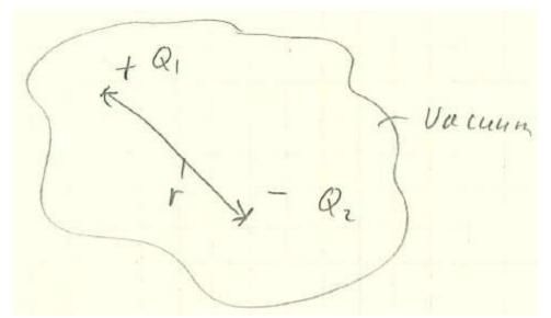
An attractive electrostatic force exists between  $Q_1$  and  $Q_2$  that attempts to bring the two charges into contact. Let that force be  $F_{EL}$ :
