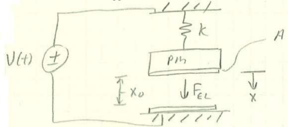
Here, the PPA has been integrated with a MEMS SMD where the proof mass is a movable electrode and the frame is a fixed electrode.
