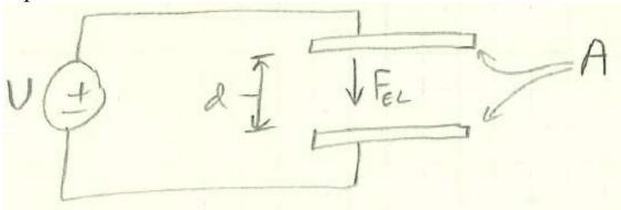
where A is the electrode surface area, d is the electrode separation distance, and V is an applied DC voltage.
