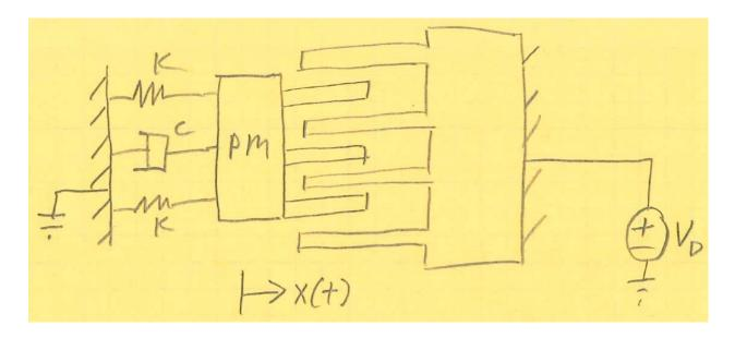
NOTE: k is the system spring constant and  $V(t) = V_D$ . Our system differential equation becomes:
