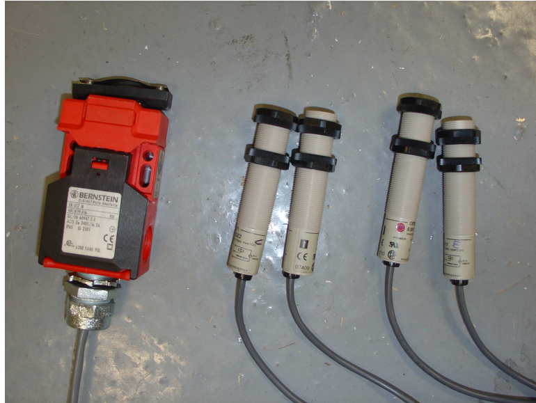
Figure 8 - Optical Sensors and Door Switch
