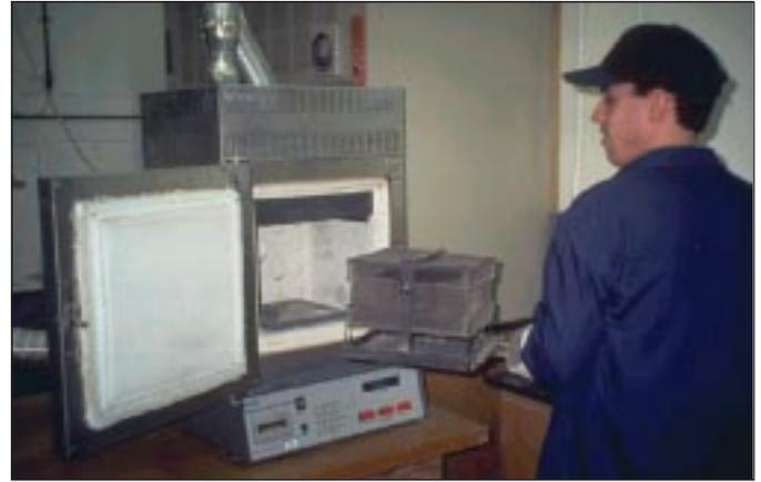
NCAT ignition oven for determining asphalt content
