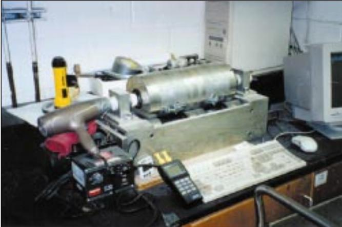
NCAT aggregate bulk specific gravity device
