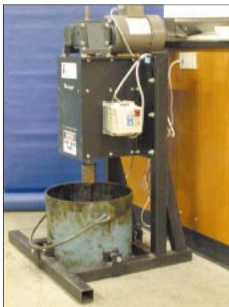
NCAT workability device for HMA
