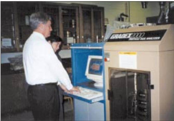
*NCAT automated aggregate gradation device*
