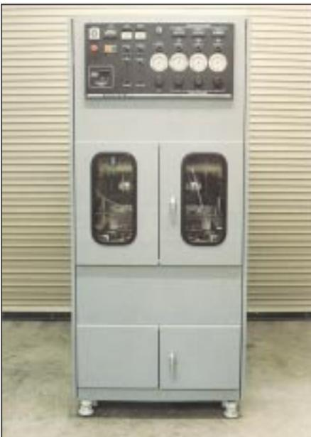
*Asphalt Pavement Analyzer*
