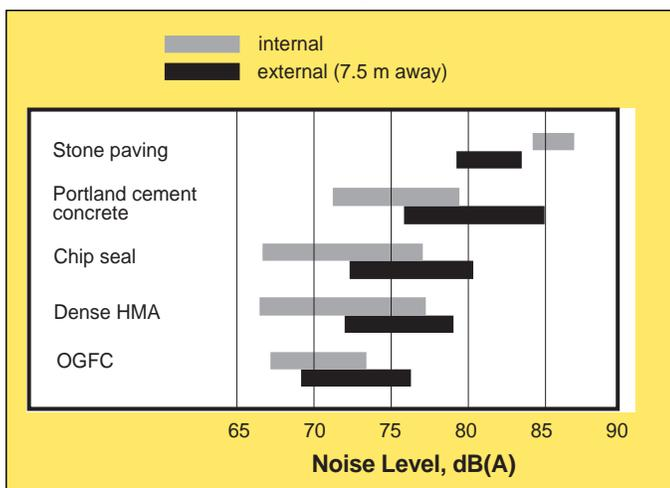
Figure 4. Variation of Tire-Pavement Contact Noise (Outside and Inside a Car at 8- km/Hour) on Various Surface Types
