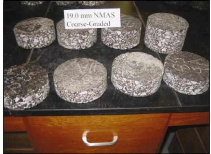
*Cores obtained from test sections which used different lift thicknesses for 19 mm coarse-graded Superpave mix*
