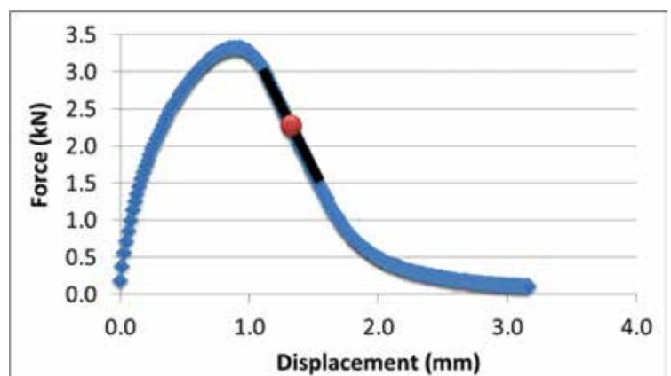
Figure 1: I-FIT Test Setup (left) and Example I-FIT Data (right) with Post-Peak Slope Highlighted
