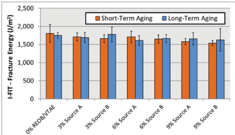
Figure 2: I-FIT Average and Standard Deviation of Fracture Energy
