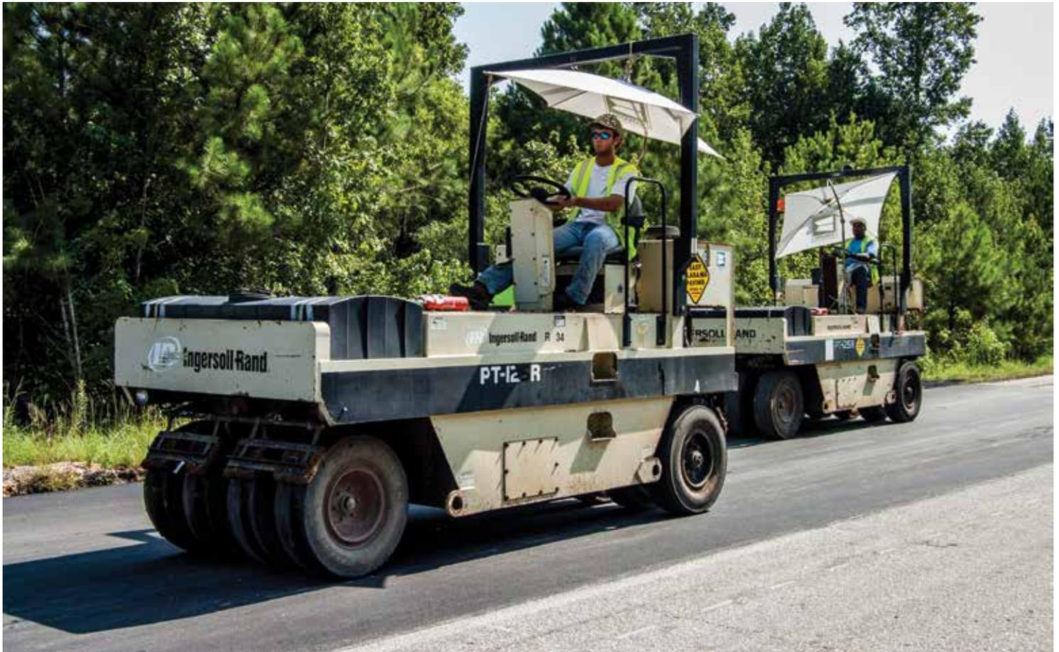
Pneumatic tire rollers are used on the NCAT Test Track to achieve proper compaction and in-place density.
