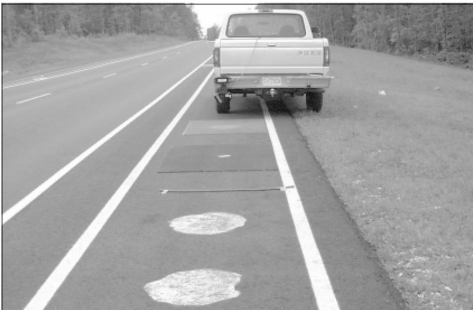
*ROSAN<sub>v</sub> laser system mounted on the bumper of a vehicle for surface texture measurements to identify segregation in HMA pavements. Sand patch method was used for evaluating surface texture for comparison.*
