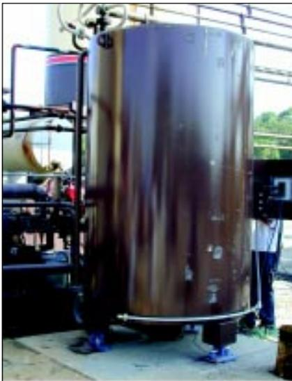
Figure 6. Asphalt meter calibration tank
