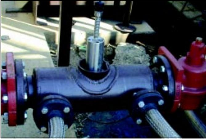
Figure 5. In-line asphalt viscometer
