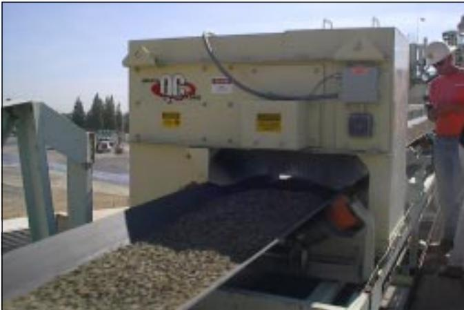
Figure 1. Automated belt sampler is used to obtain a sample of the material rapidly from the moving conveyor belt
