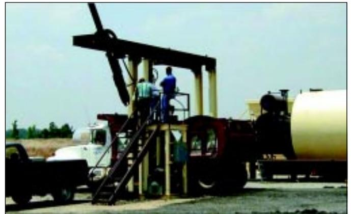
Figure 7. Robotic truck sampler
