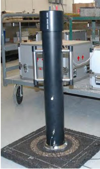
Figure 3 Impedance Tube
