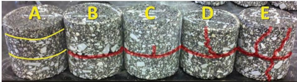
Figure 22 (b) Cores Taken from Section S5 (High RAP) in April 2013 (Cracks and Debonding Highlighted)
