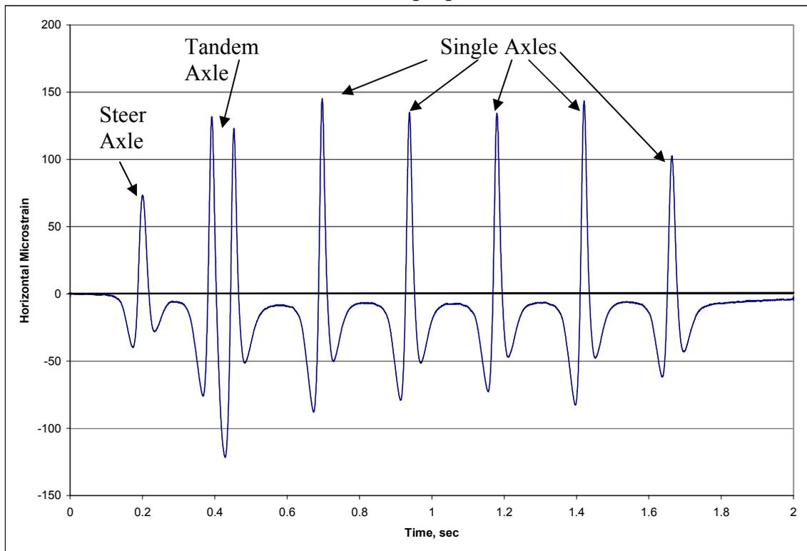
Figure 4.1 Longitudinal Strain Trace – Example 1.
