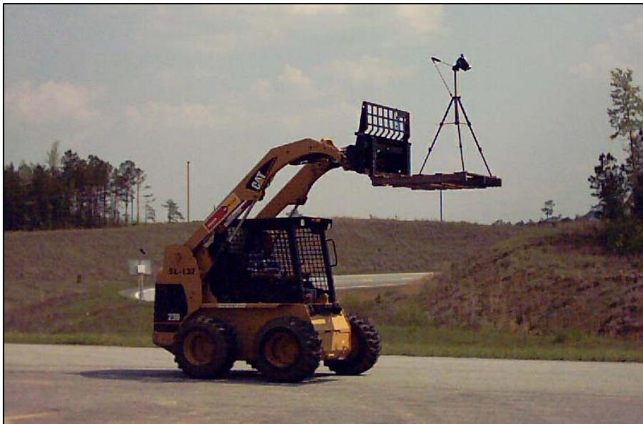
Figure 3.10 Camera Apparatus for Crack Record.
