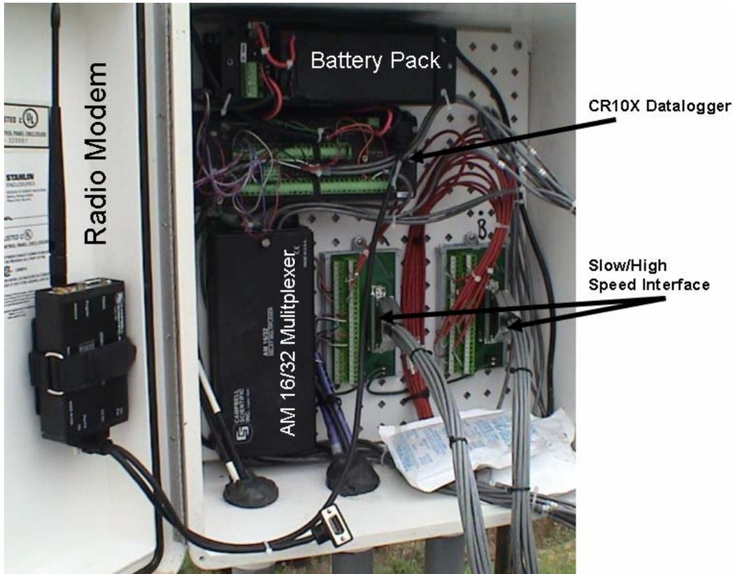
Figure 3.5 Roadside Box and Datalogger (Timm et al., 2004).
