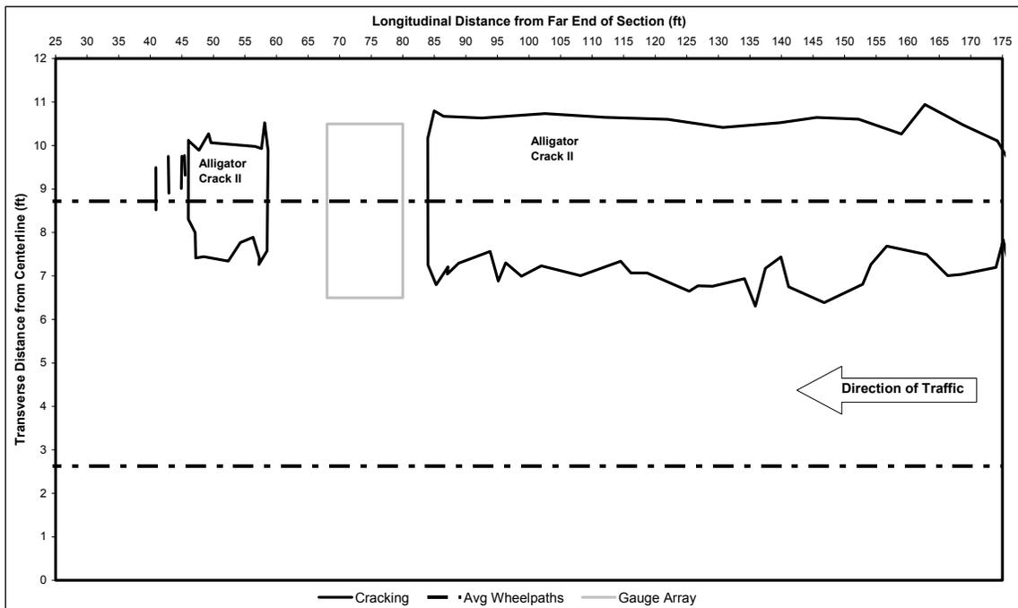
Figure 5.23 N2 Crack Map 8/02/2004.
