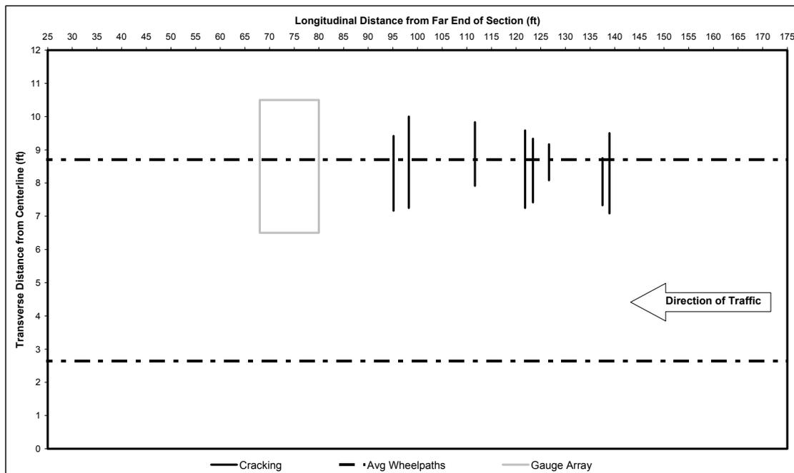
Figure 5.21 N2 Crack Map 6/21/2004.
