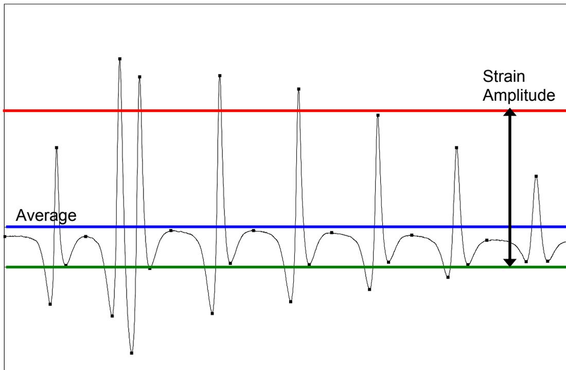
**Figure 4.7 Strain Amplitude Illustration – Example 1.**
