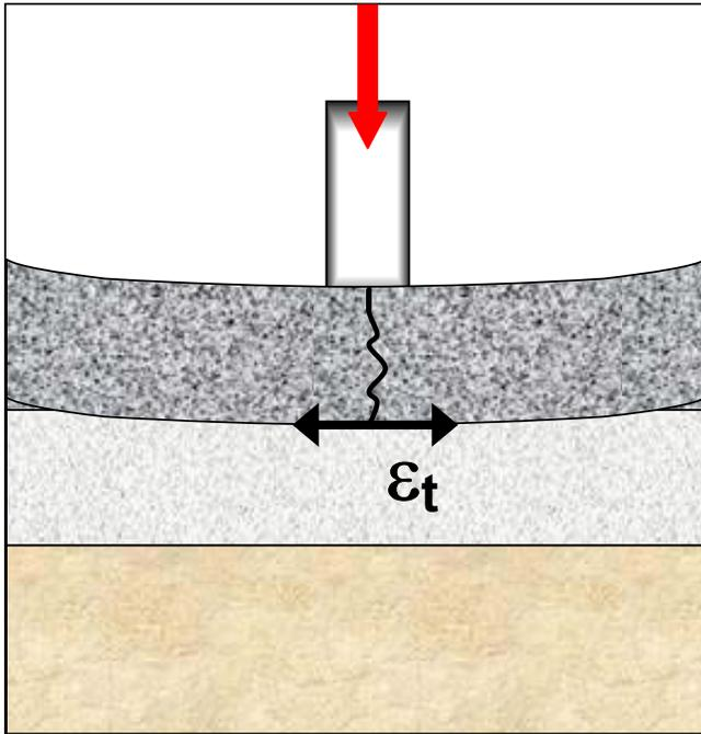
**Figure 2.2 Schematic of Fatigue Cracking Mechanism in Pavement Cross Section.**
