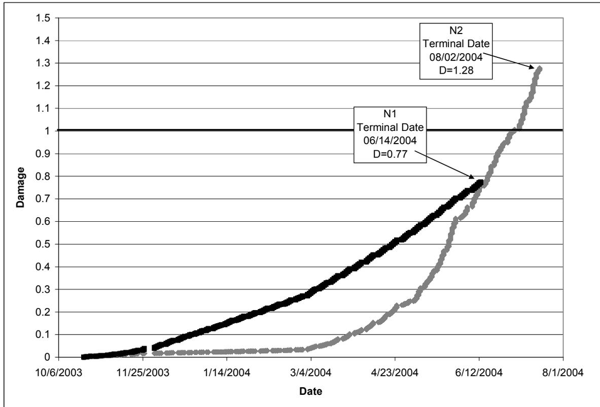
**Figure 6.2 Damage Accumulation for Sections N1 and N2.**
