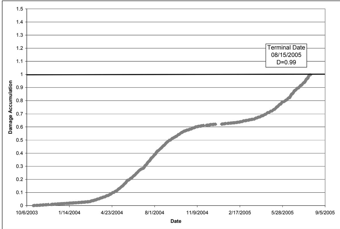
**Figure 6.5 Damage Accumulation for Section N8.**
