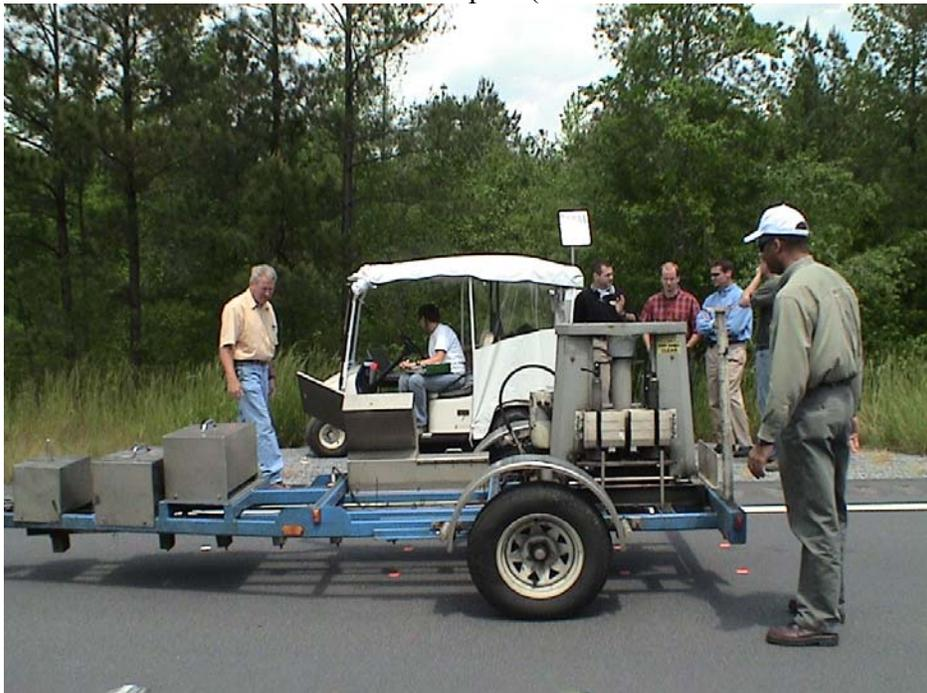
**Figure 3.8 FWD Testing and Data Collection.**
