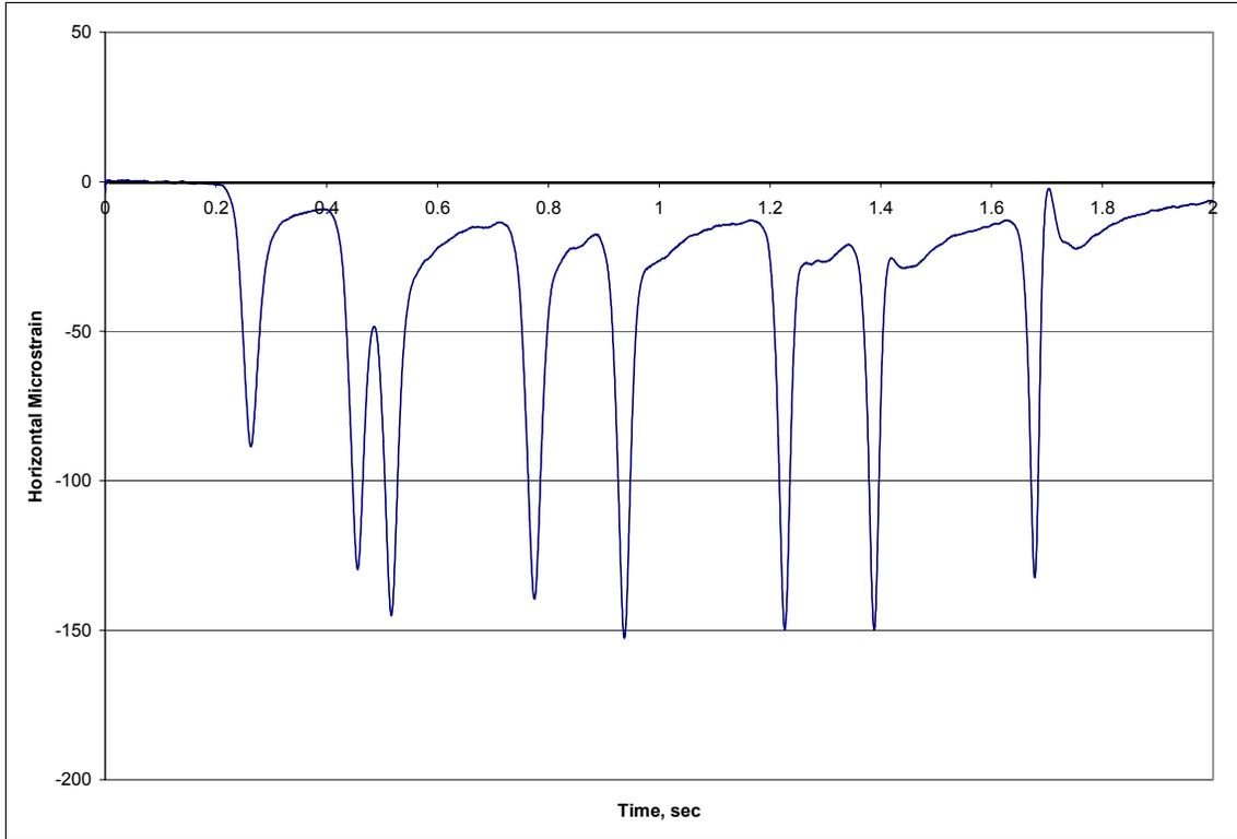
Figure 4.3 Transverse Strain Trace – Example 1.
