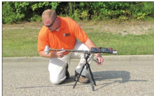
Figure 1 Measuring solar reflectance with a pyrometer according to ASTM E 1918.
