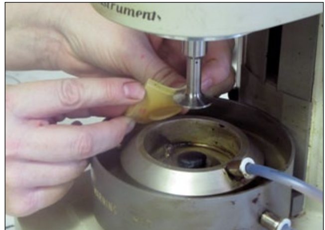
Figure 1 The Steady Shear Flow and Phase Angle methods use a standard dynamic shear rheometer (DSR).
