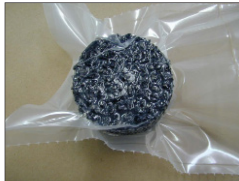
Figure 1 Sealed HMA sample following the Corelok procedure.
