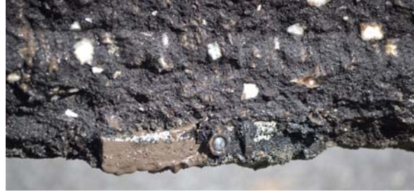
a) Embedded Gauge in Slab from Trench 2
