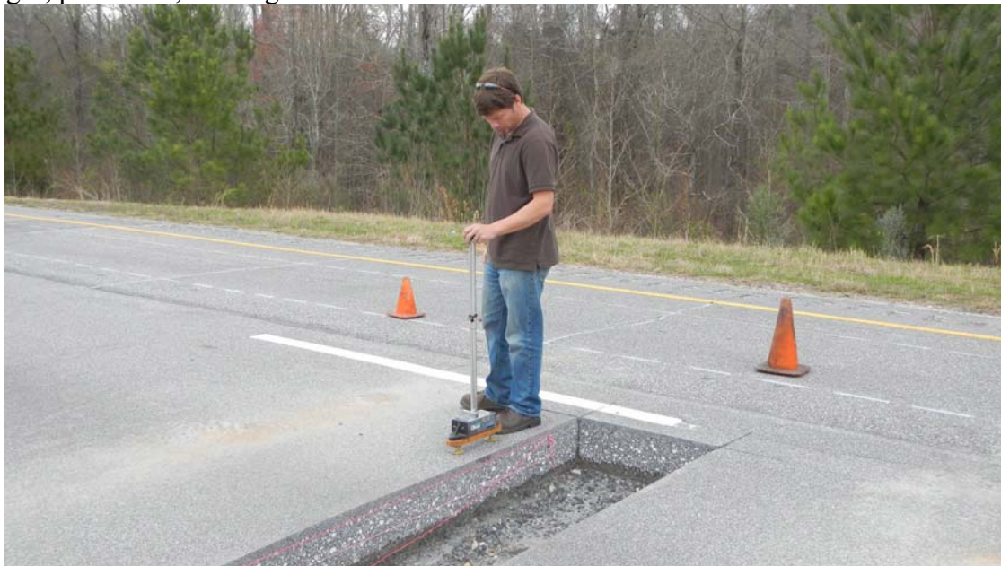
Figure 5.9 Walking Dipstick at Surface
