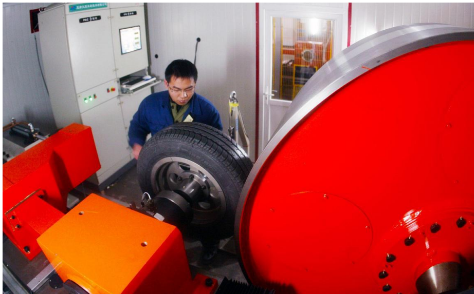
Figure 4.1 Drum Type Tire Test ( http://jiurongwheel.com )
