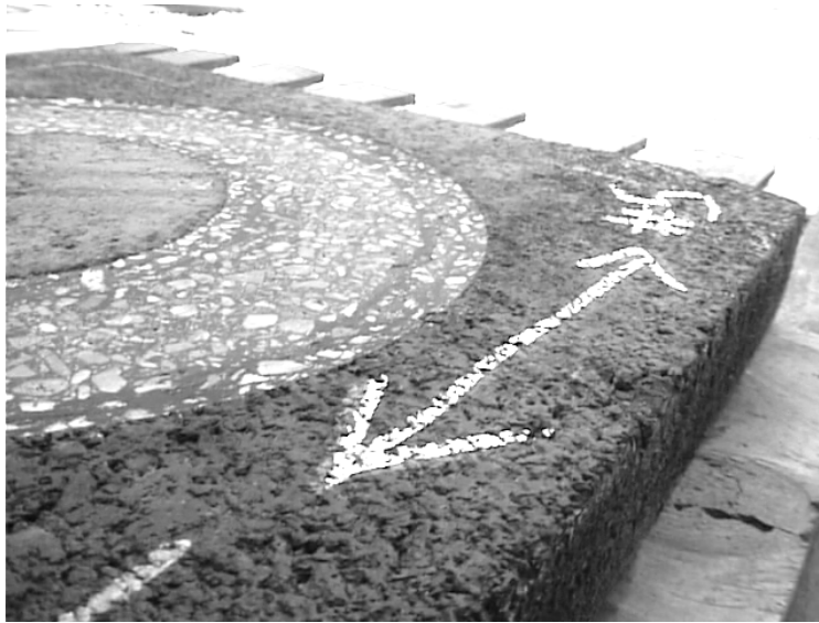
Figure 27. Abrasion of Surface by Steel Wheel
