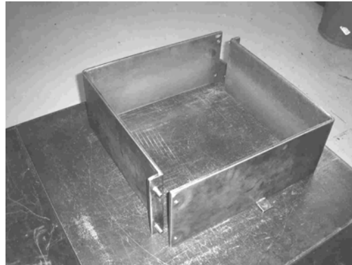
Figure 13. New 20" by 20" Mold for Hamburg Compactor
