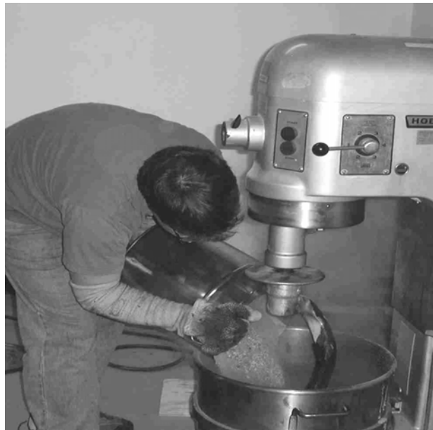
Figure 6. Mixing Aggregates Prior to Adding Asphalt Cement
