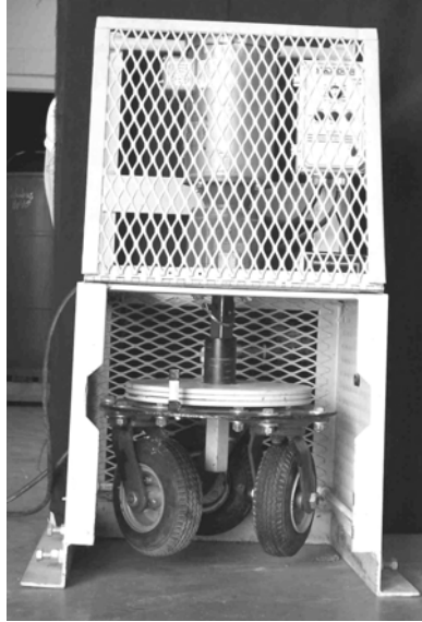
Figure 25. Slab Placed in Slotted Area at Bottom of Polishing Machine
