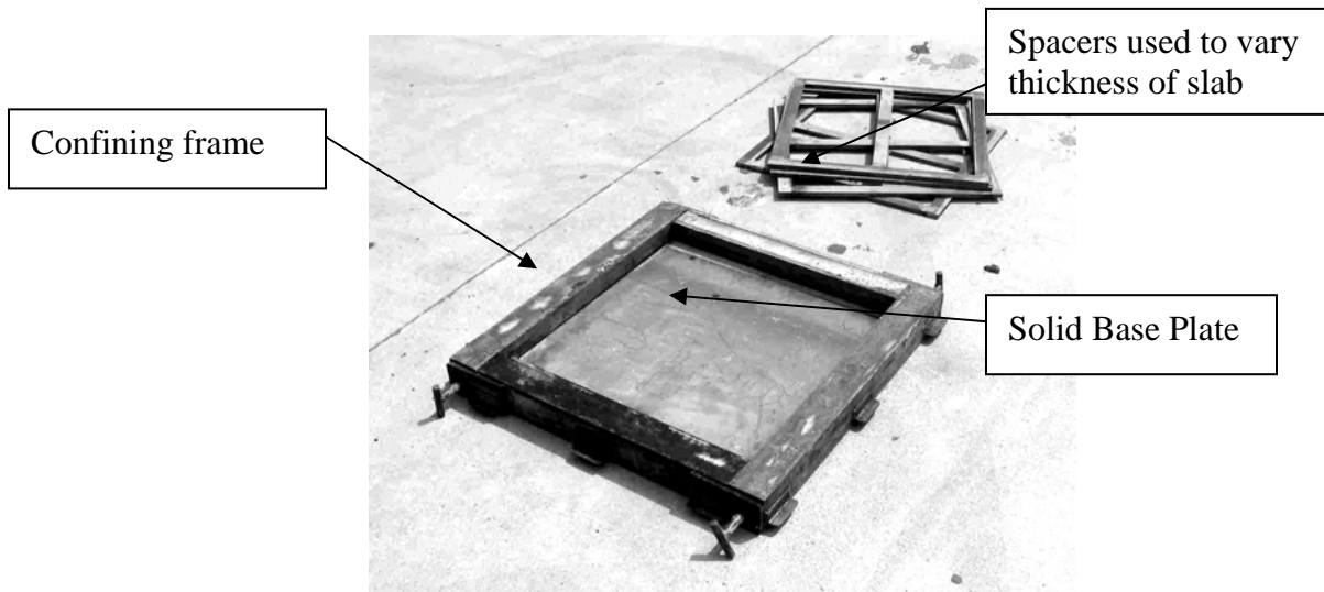
Figure 8. Square Mold (24'' by 24'') with Solid Base Plate
