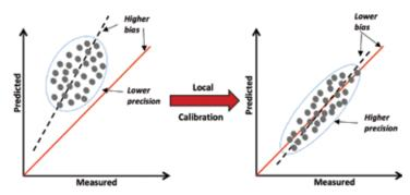
Figure 1: Improvement of Bias and Precision through Local Calibration
