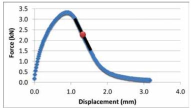
Figure 1: I-FIT Test Setup (left) and Example I-FIT Data (right) with Post-Peak Slope Highlighted
