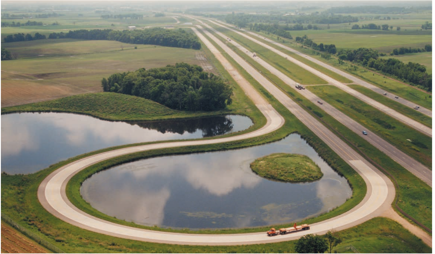
An 80,000 pound five-axle tractor-trailer operates on MnROAD's closed loop adjacent to Interstate 94 (I-94).
