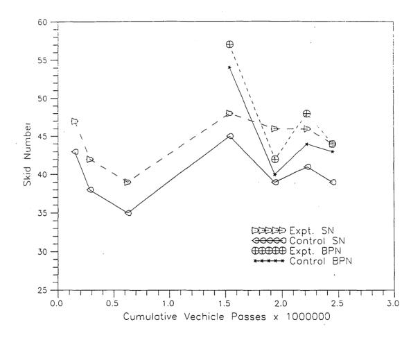
Figure 3. SN versus cumulative vehicle passes (Chilton County)
