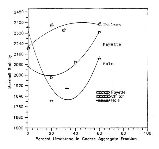
Figure 1. Marshall stability versus percent limestone in the coarse aggregate fraction.
