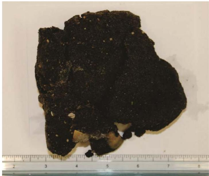
**Figure 3.** Submerged tar mat sample collected from surf zone immediately after Tropical Storm Lee (scale in inches; collected September 8, 2011).
