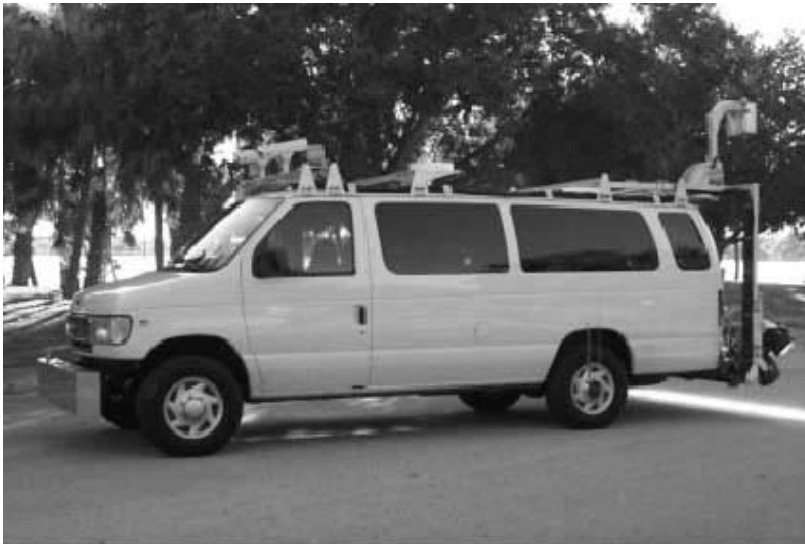
Figure 2.4 Automated Pavement Condition Survey Vehicle (ICC, 2003).
