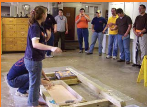
Students in the department demonstrate a non-newtonian fluid pool, a liquid polymer that can be used in protective gear for the military
