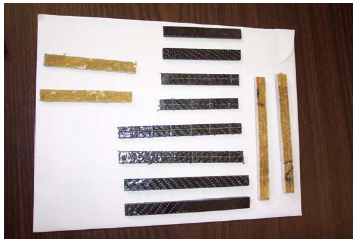
Figure 5 Preparation of samples for 3 point bending tests
