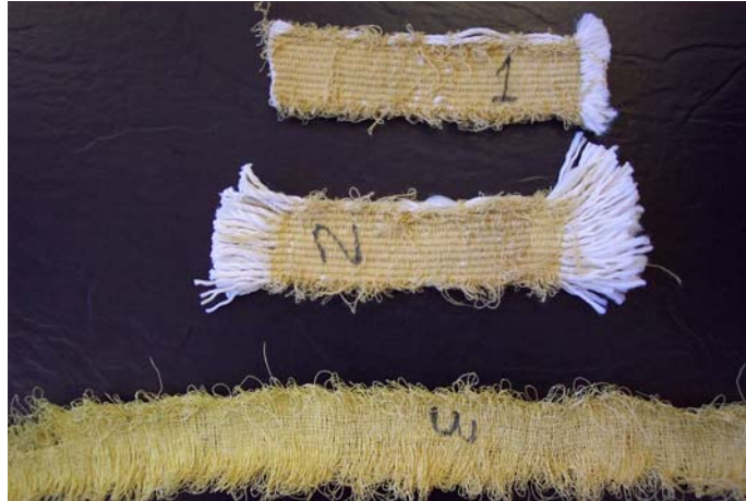
Figure 2. Examples of 3D hybrid woven/knit preforms produced
