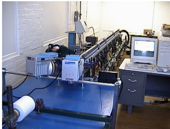
Figure 1 Air-jet filling insertion simulator developed at Auburn University
